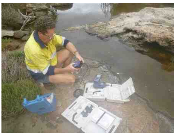
Plate 1. Field Sampling of in situ water quality using WTW meters.
