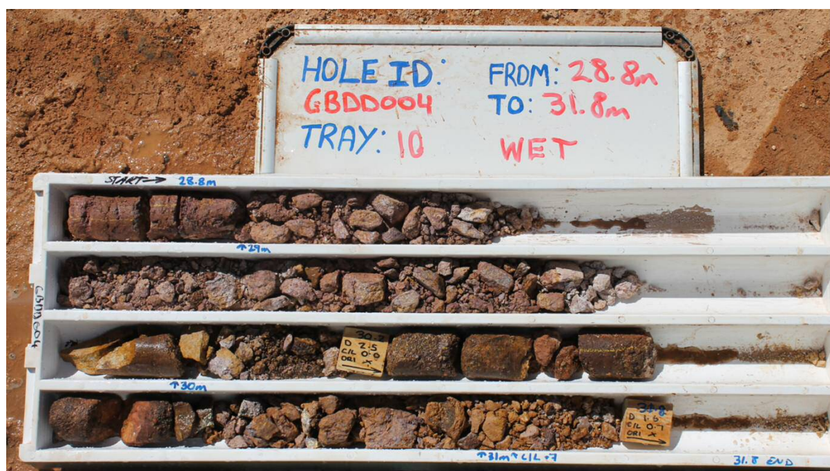
Figure 4.4: Core from GBDD004 showing unconsolidated gravel and pisolite
