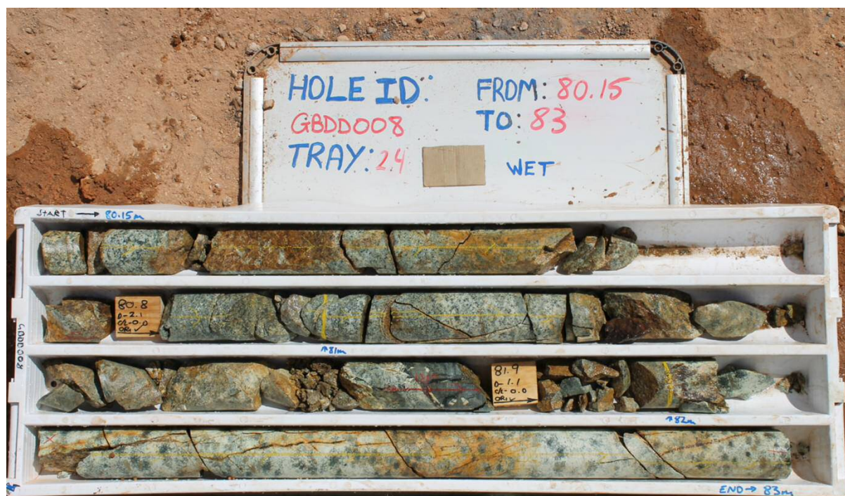
Figure 4.3: Core from GBDD008 showing stained fracture zones at depth
