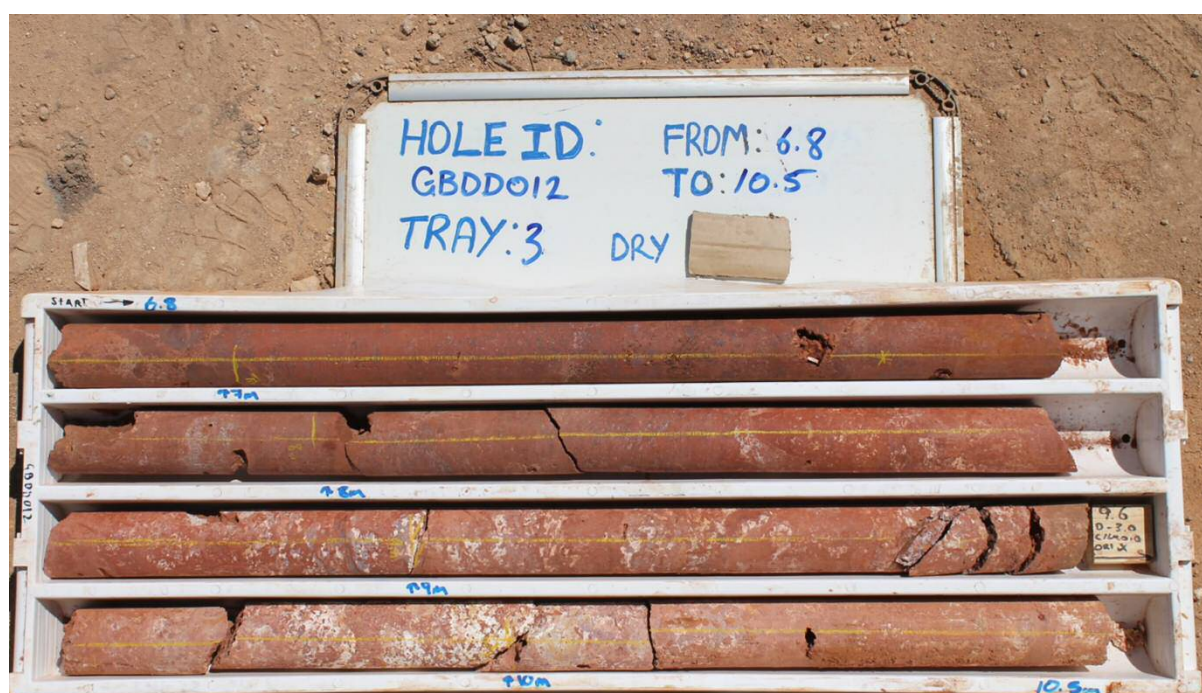
Figure 4.2: Core from GBDD012 showing pores/ cavities from secondary weathering
