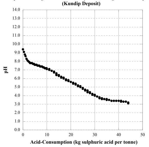
Note: The  $H_2SO_4$ -addition rate employed in the auto-titration corresponds to a sulphide-oxidation rate (SOR) of c. 2-3 x  $10^5$  mg  $SO_4$ /kg/week (= c. 1-2 x  $10^4$  kg  $H_2SO_4$ /tonne/year).
