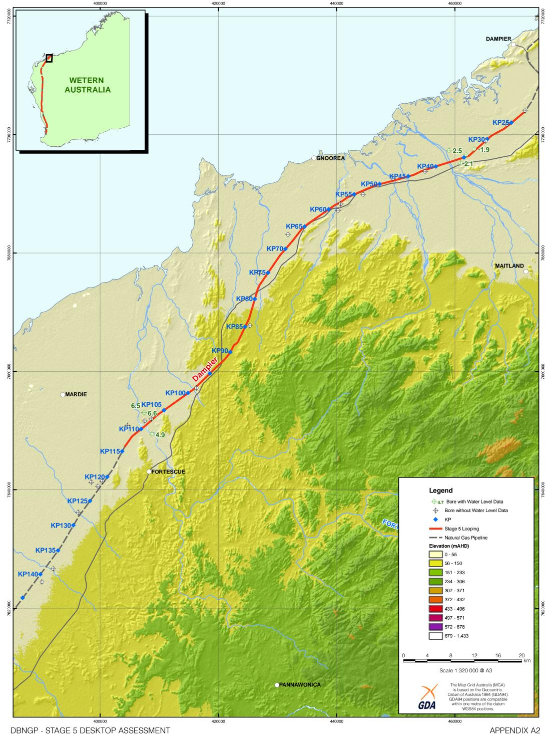
LOOPING 0 (DAMPIER) - TERRAIN AND DEPTH TO GROUNDWATER (mBGL)
