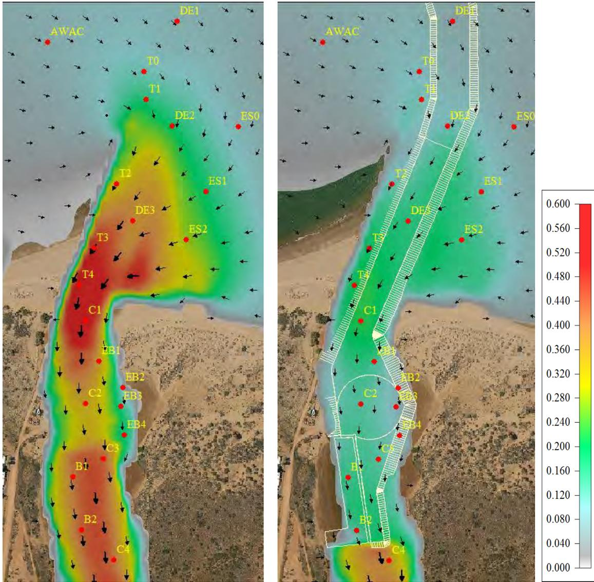
**Figure 5.8: Comparisons of depth averaged current speed through Beadon Creek entrance during a large flood tide for the existing (left) and developed (right) case (1 October 2015 1100 WST).**
