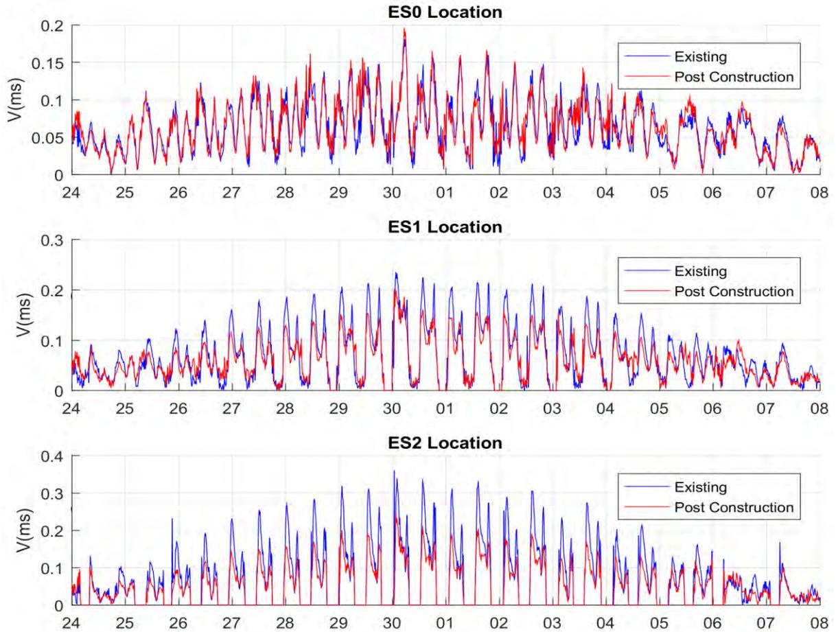
**Figure 5.13: Modification to flow velocities on the eastern shoal post construction (Spring Tide 24 Sep to 8 Oct 2015)**
