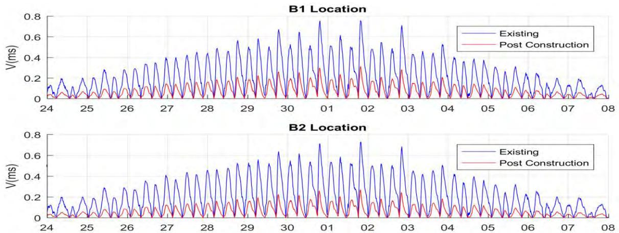
**Figure 5.16: Flow velocities during the neap-flood phase in the Berth Pocket Post Construction (Spring Tide 24 Sep to 8 Oct 2015)**
