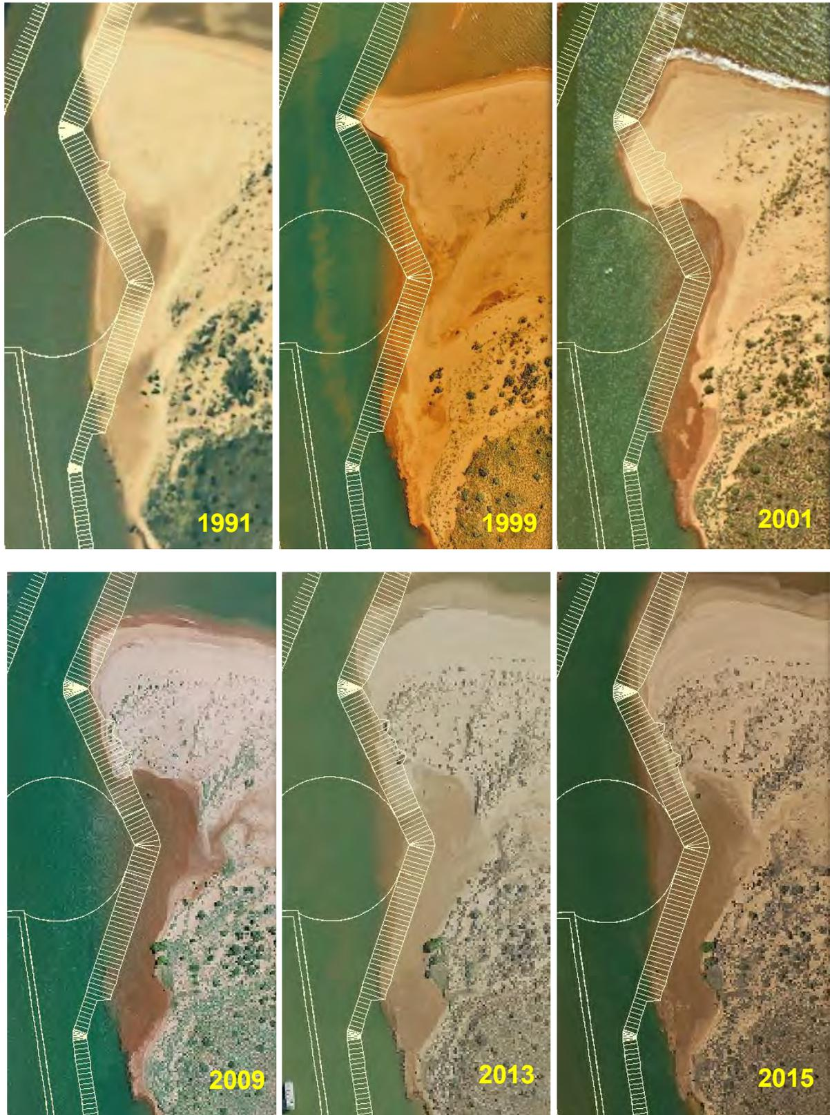
Figure 6.6: Eastern shoreline with aerial imagery overlain with proposed dredge area footprint for years 1991, 1999 (post cyclone TC Vance), 2001, 2009 (post TC Dominic), 2013 and 2015.
