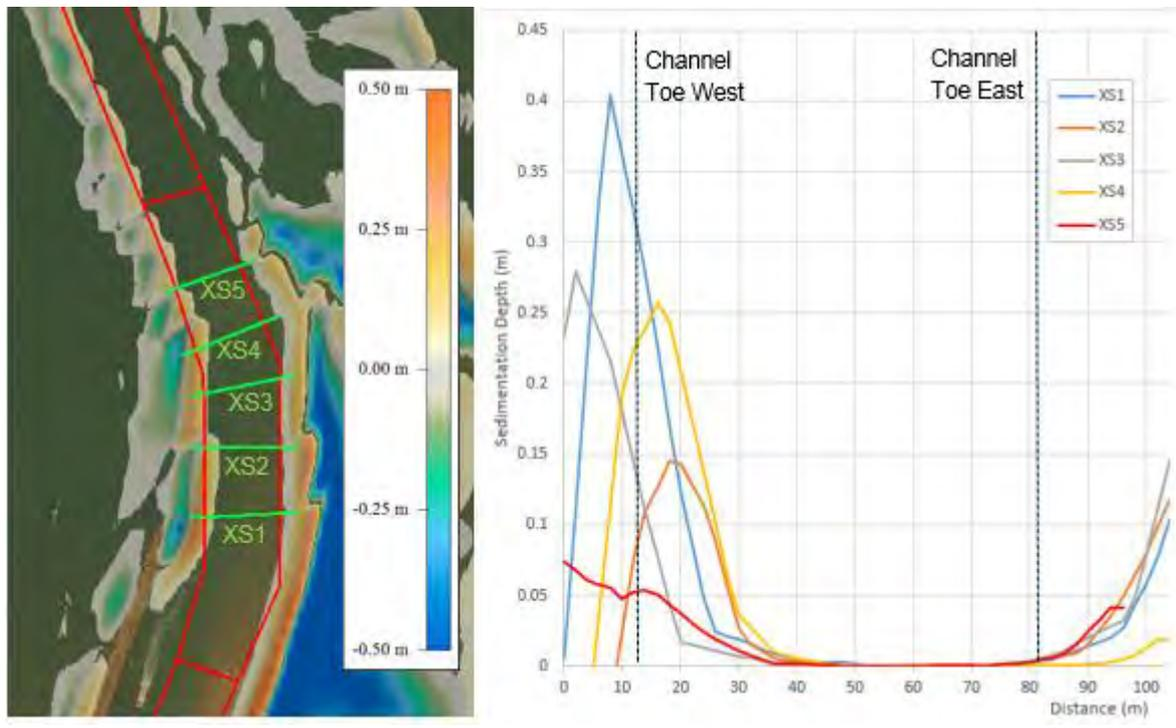
**Figure 6.21: Modelled sedimentation for cross sections through the channel approach (section 2)**
