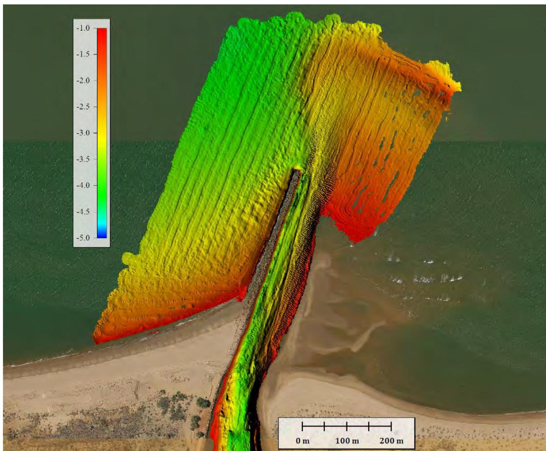
**Figure 6.5: Multi-beam bathymetry showing seabed elevation at the Beadon Creek Entrance (Datum m AHD)**
