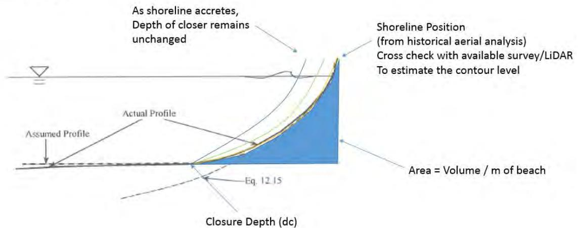
**Figure 6.8: Schematic of Cross Shore Profile Analysis based on the equilibrium profile concept in Kamphuis (2010)**
