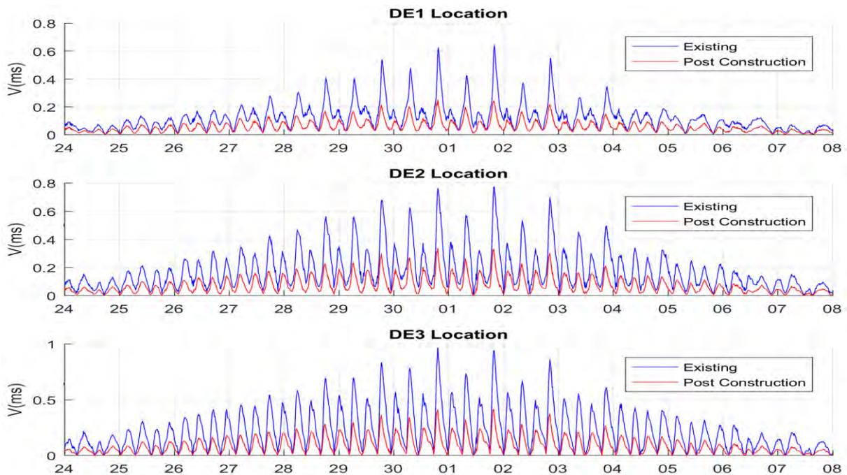
**Figure 5.17: Flow velocities during the neap-flood phase in the Main Access Channel Post Construction (Spring Tide 24 Sep to 8 Oct 2015)**
