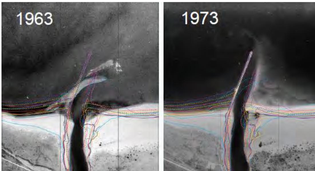
**Figure 6.1: Historical aerials showing construction of the training wall on the western sand spit at the entrance to Beadon Creek (Seashore 2017)**
