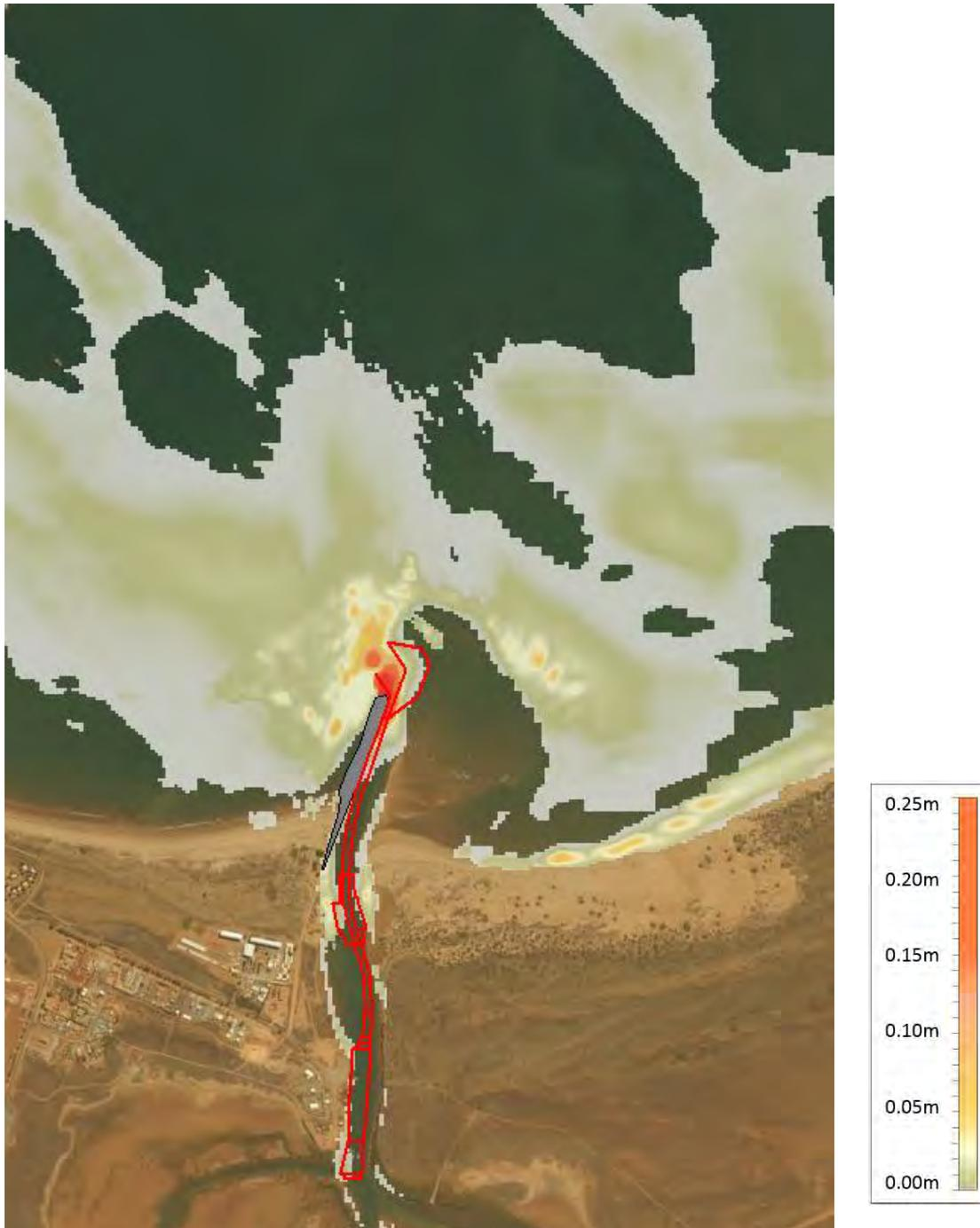
**Figure 6.25: Distribution of Littoral Drift Volume that Bypasses the Training Wall Structure under existing conditions**
