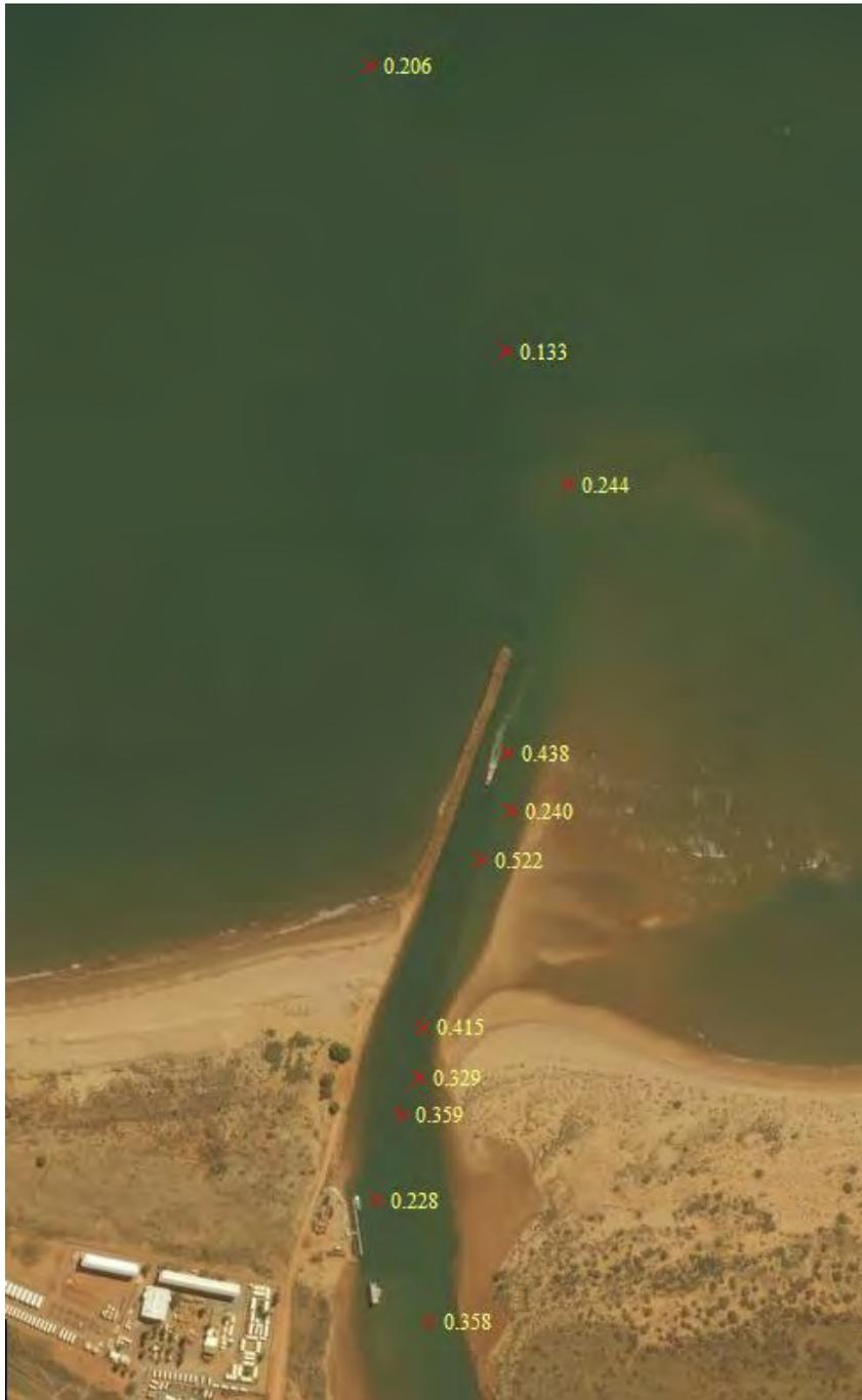
**Figure 6.15: Results for sediment size ( $D_{50}$ , mm) at sampling locations in the Entrance Channel (O2 2017) used for the discretisation in Delft3d Model Map of variable sediment size.**
