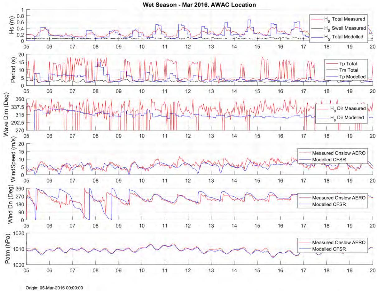
**Figure 6.14: Wet season comparison of measured and modelled wave, wind and atmospheric pressure conditions**
