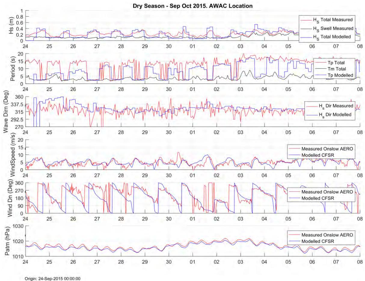
**Figure 6.13: Dry season comparison of measured and modelled wave, wind and atmospheric pressure conditions**
