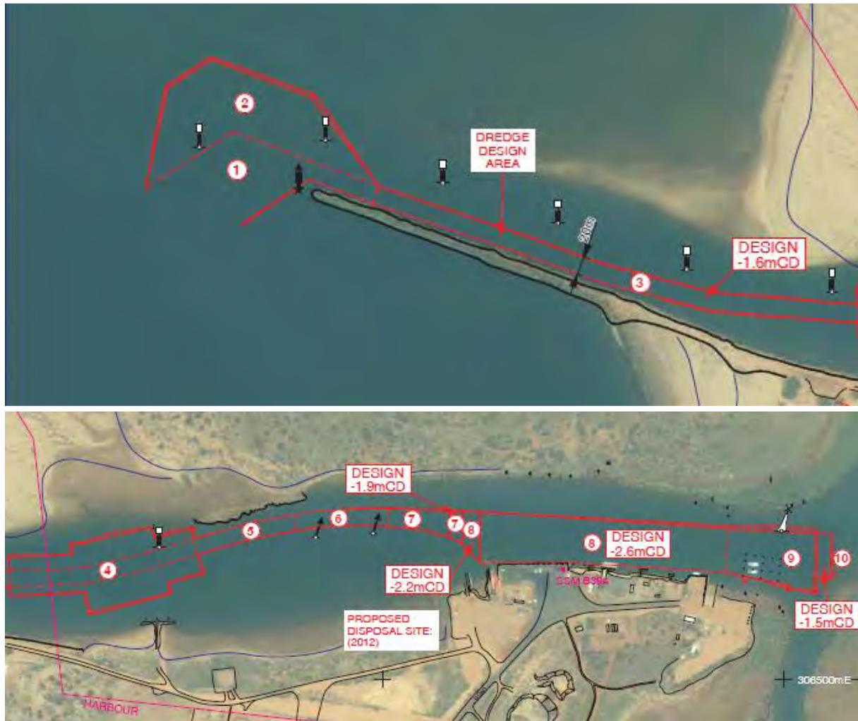
**Figure 6.17: Channel sections analysed for bed level changes (Oceanica, 2014)**
