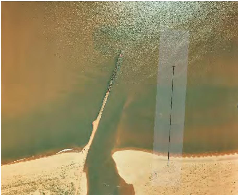
**Figure 6.12: Example of suspended fine sediments at the Beadon Creek entrance (image 1991)**
