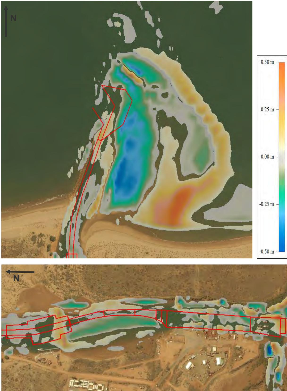
Figure 6.18: Sand fraction modelled annual erosion and sedimentation for the existing case. Outer channel (upper) and inside Beadon Creek (lower) areas with channel sections overlaid.
