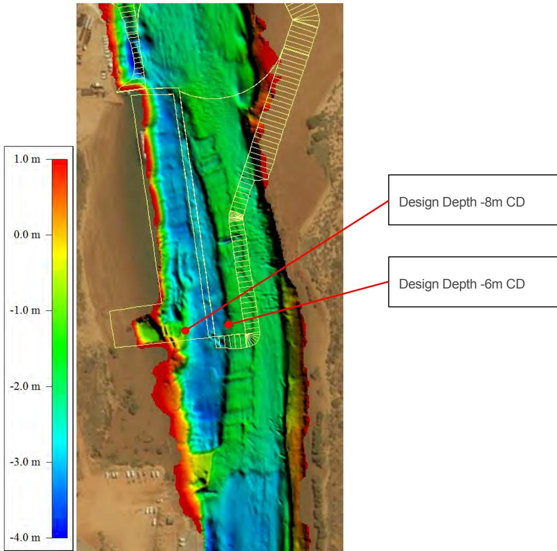
**Figure 6.22: Depth transition through from the lower section of the dredged footprint to the existing seabed level of Beadon Creek (levels shown to mCD).**
