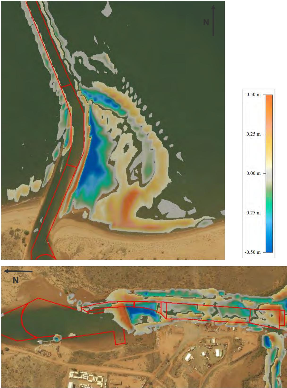
Figure 6.19: Sand fraction modelled annual erosion and sedimentation for the developed case. Outer channel (upper) and inside Beadon Creek (lower) areas with channel sections overlaid
