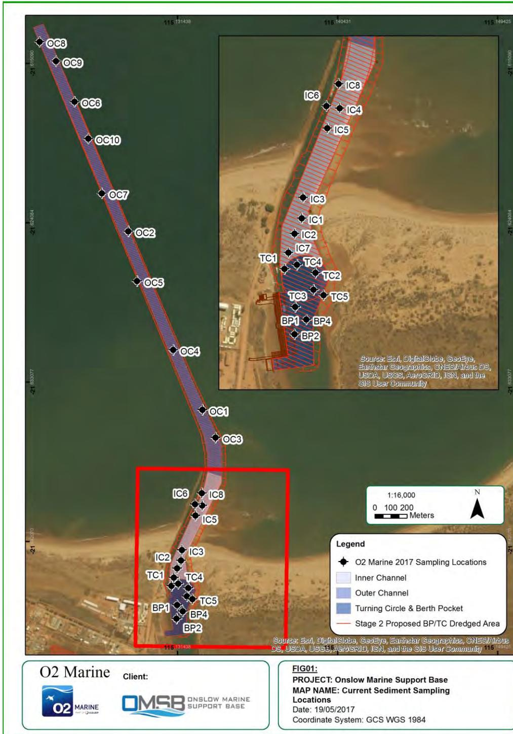
Figure 3.2: Sediment Sampling Locations (O2 Marine 2017)
