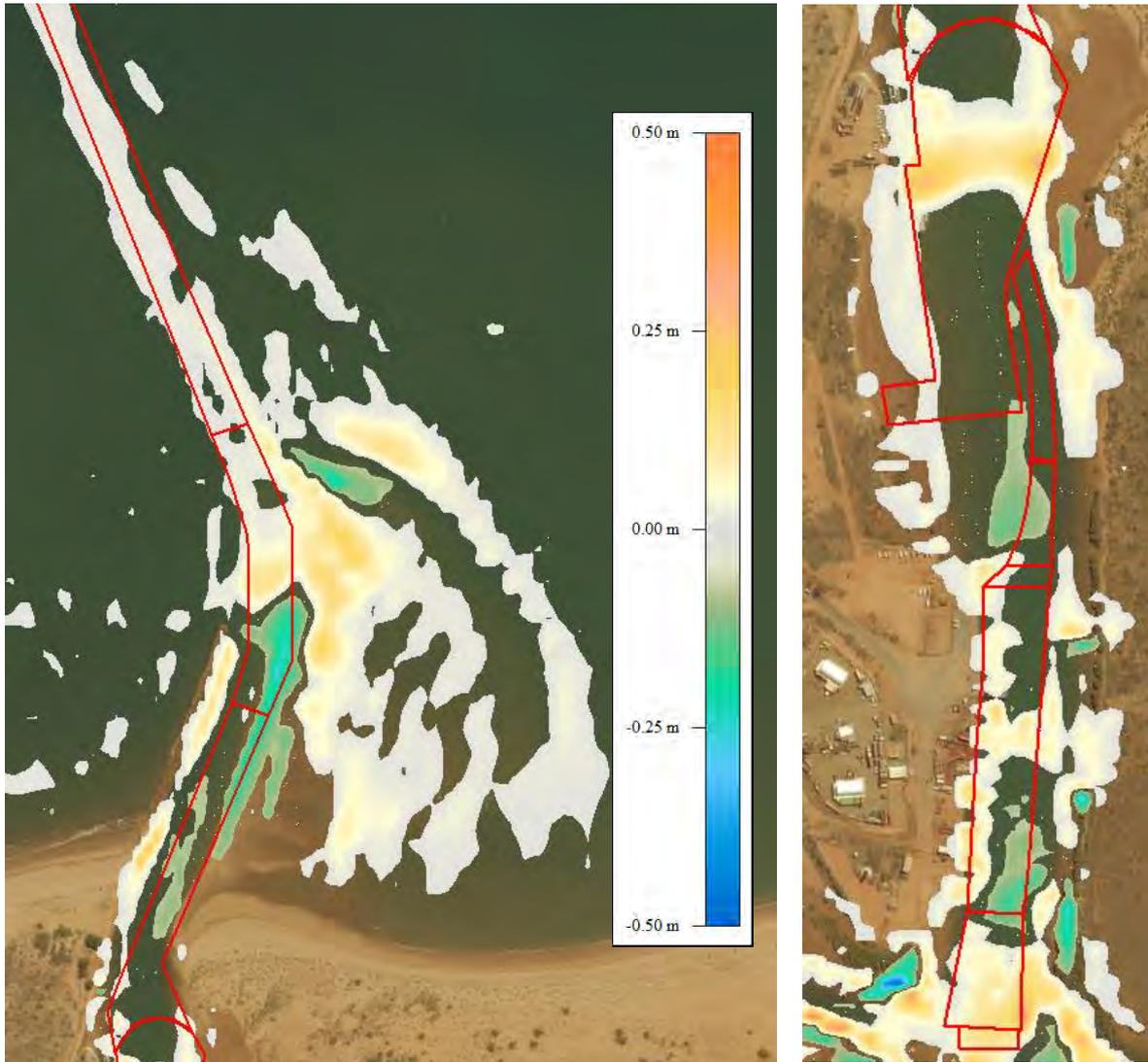
**Figure 6.31: TC Vance 1999, Sand fraction modelled erosion and sedimentation for the developed case. Outer channel (left) and inside Beadon Creek (right) areas with channel sections overlaid.**
