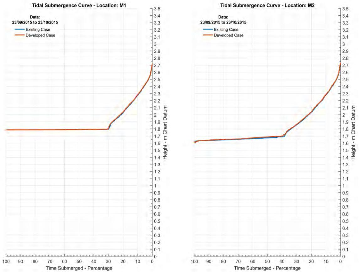
**Figure 5.20: Submergence Curve for the Mangrove Location M1 and M2 for the existing and post construction scenario**
