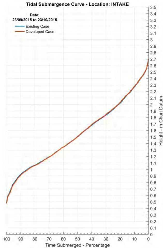
**Figure 5.18: Submergence Curve for the Salt Intake location for the existing and post construction scenario**
