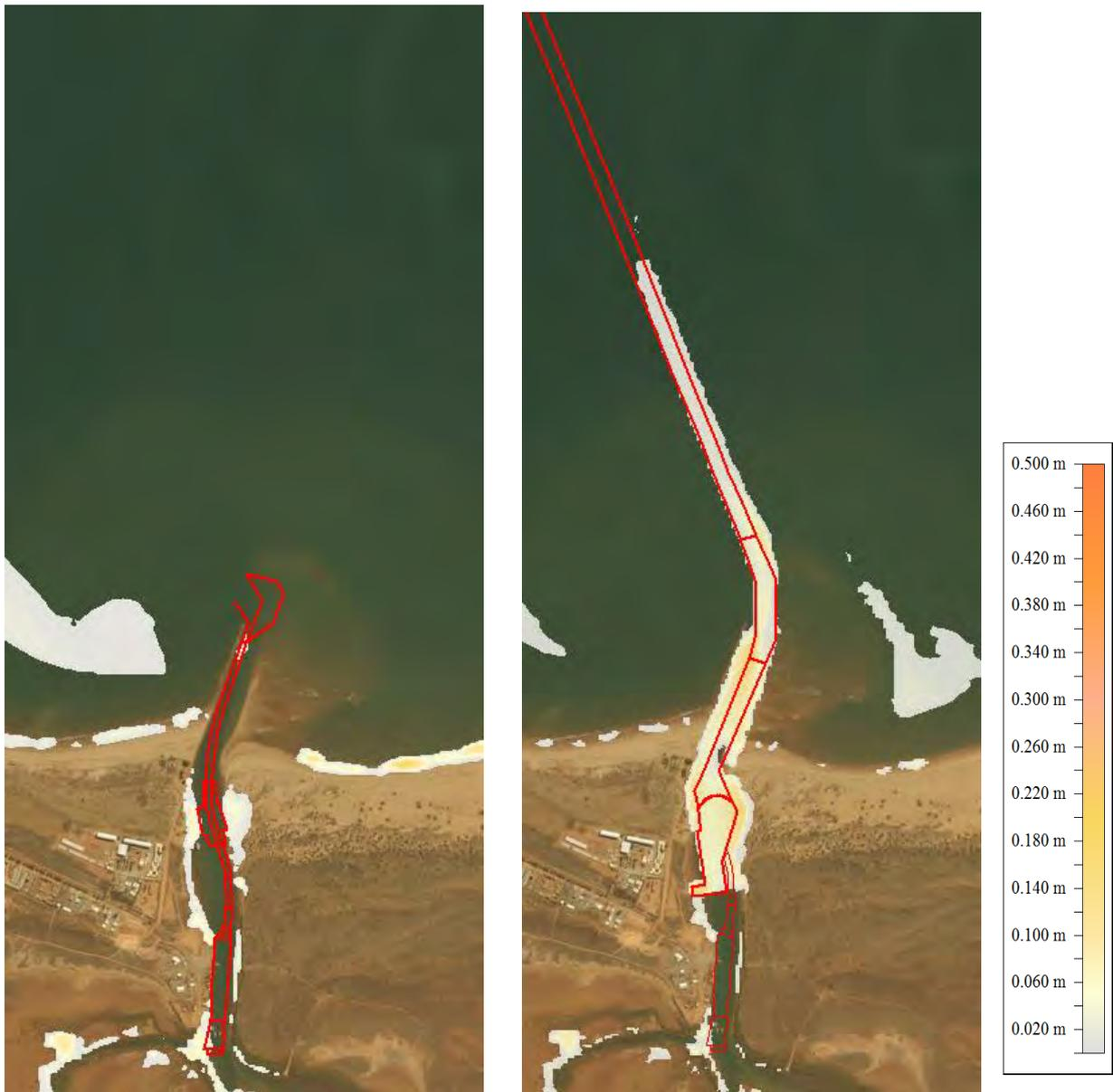
**Figure 6.23: Fines Accumulation – total annual sedimentation for Existing Case (left), Developed Case (right)**
