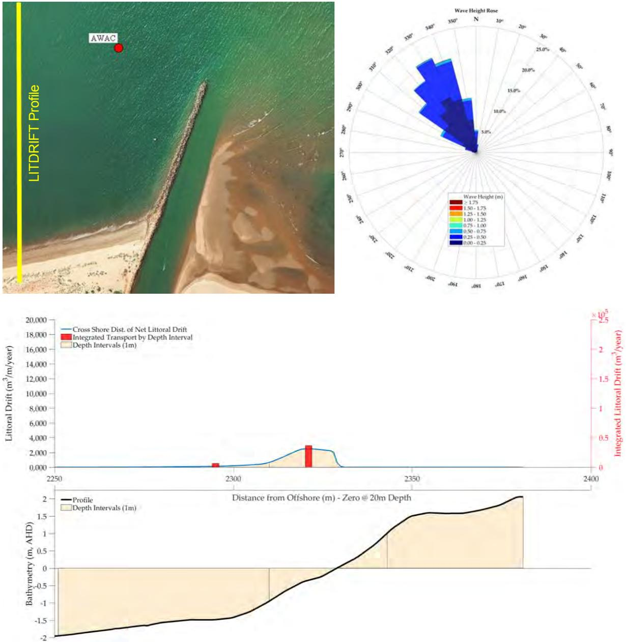
**Figure 6.7: Littoral transport modelling for the western shoreline using the LITDRIFT model.**
