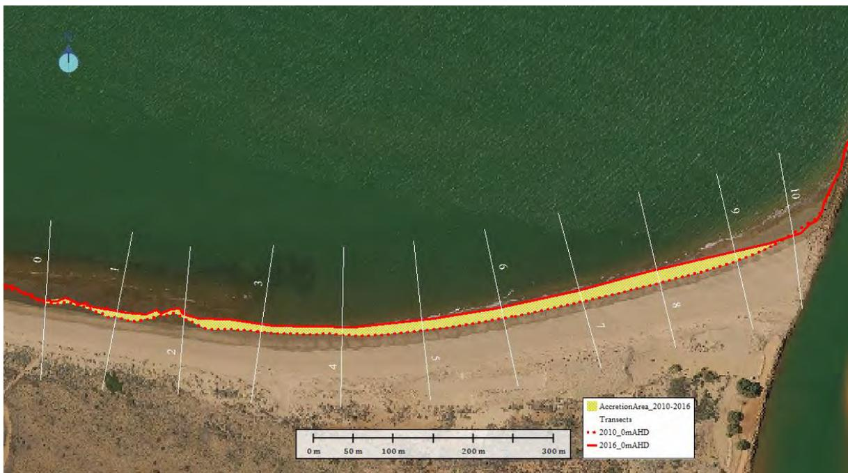
**Figure 6.9: Assessment of shoreline change based on 2010 and 2016 LiDAR**
