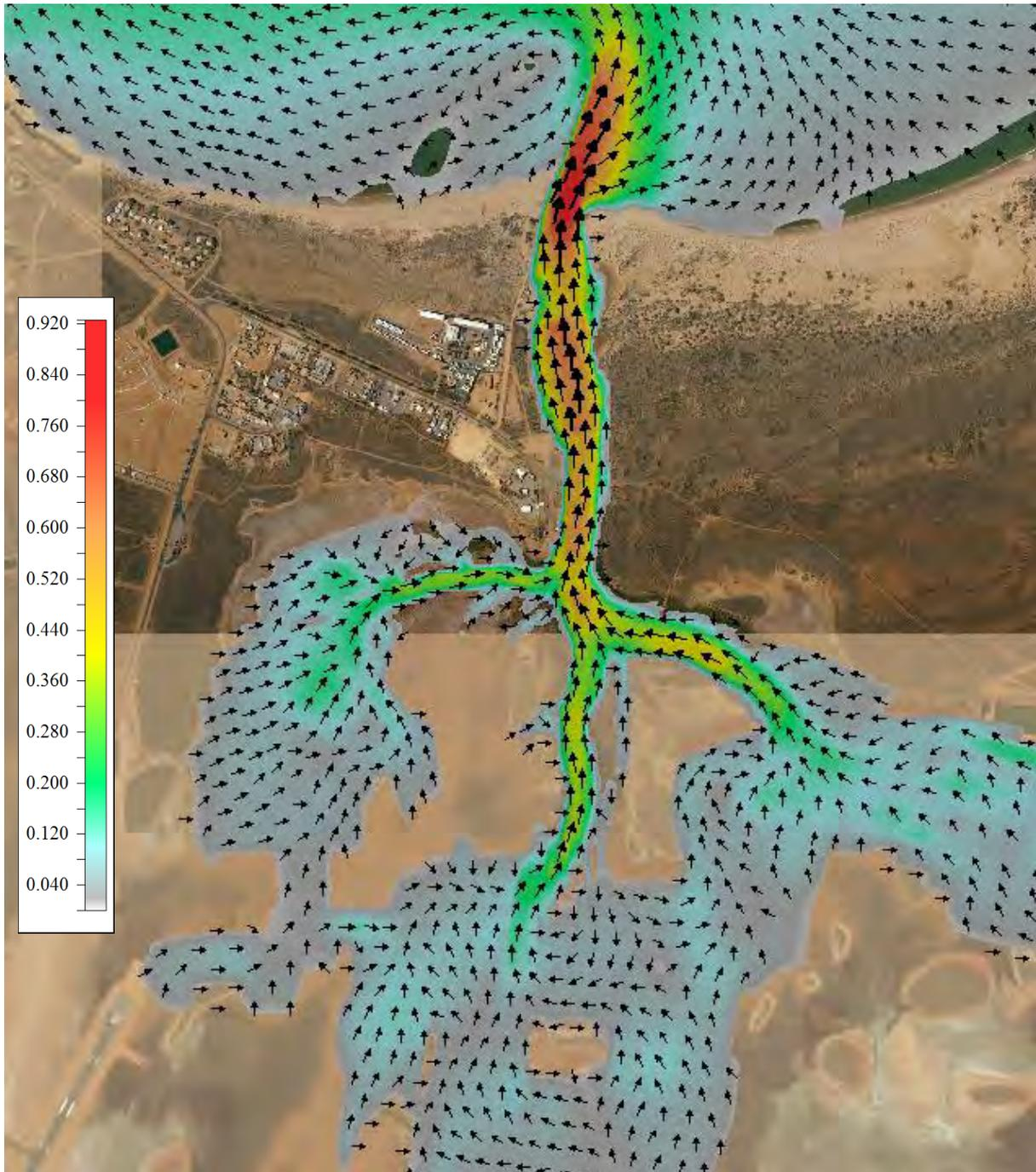
**Figure 5.9: Existing condition modelled depth average current speed through the Entrance Channel during a large ebb tide (1 October 2015 0230 WST).**
