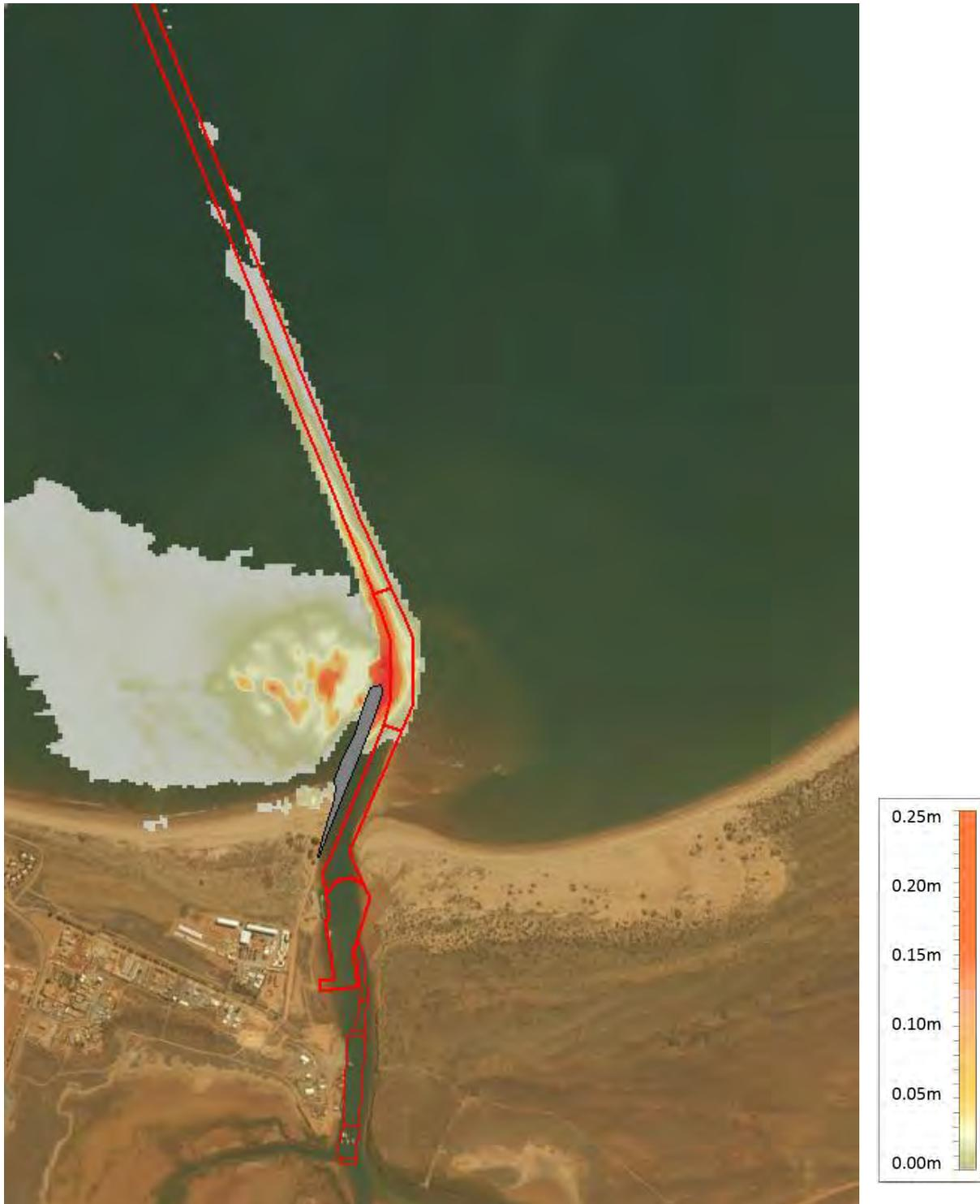
**Figure 6.26: Distribution of Littoral Drift Volume that Bypasses the Training Wall Structure under developed conditions**
