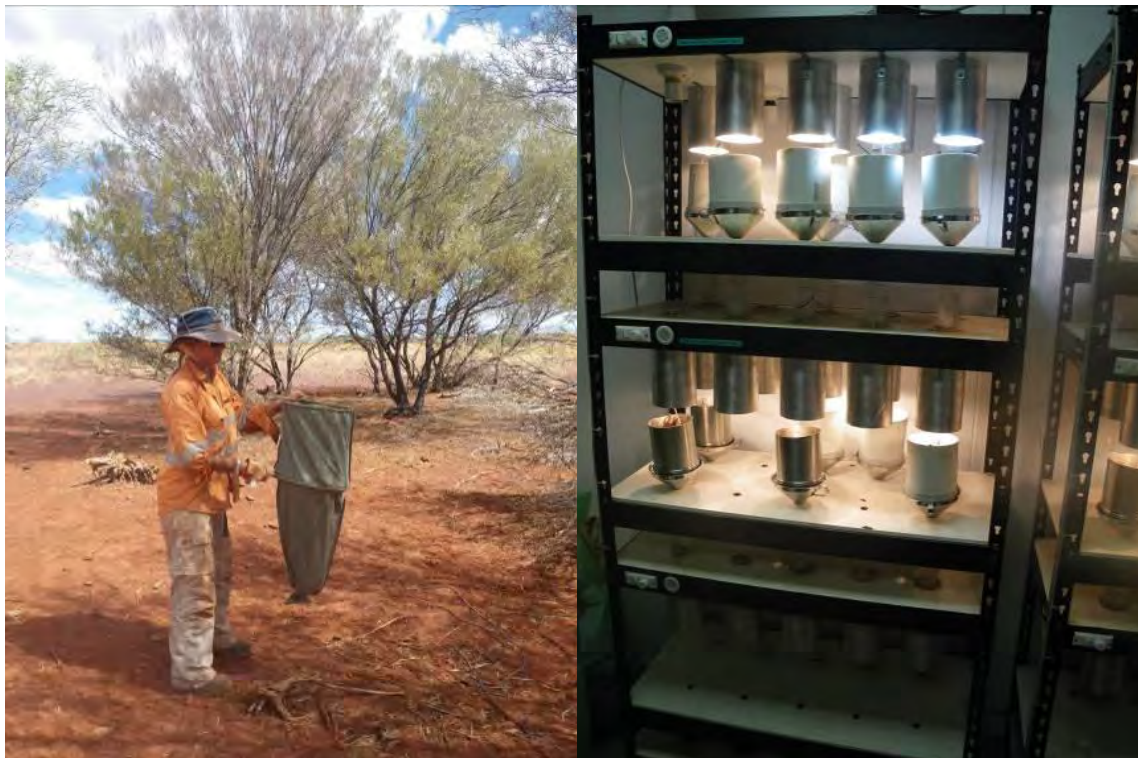
Figure 3.4 – Example of the leaf litter reducer and Tullgren funnels
