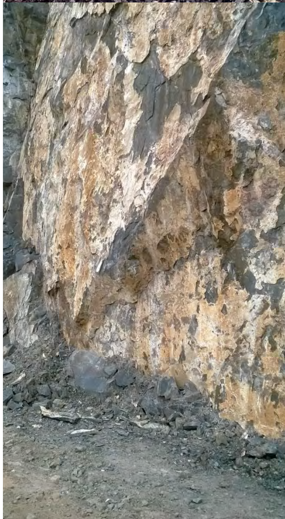
Large joint planes in the amphibolite are filled by a 2~3mm layer that fizzed vigorously in response to the 10% HCL solution.
