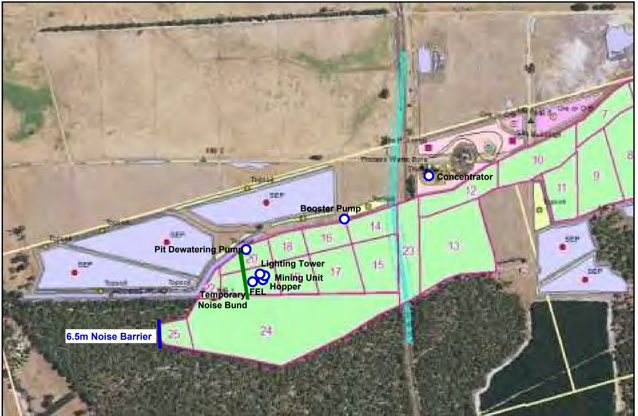
Figure 7: Assumed operating locations of the fixed plant and mobile equipment for night-time scenario 3.
