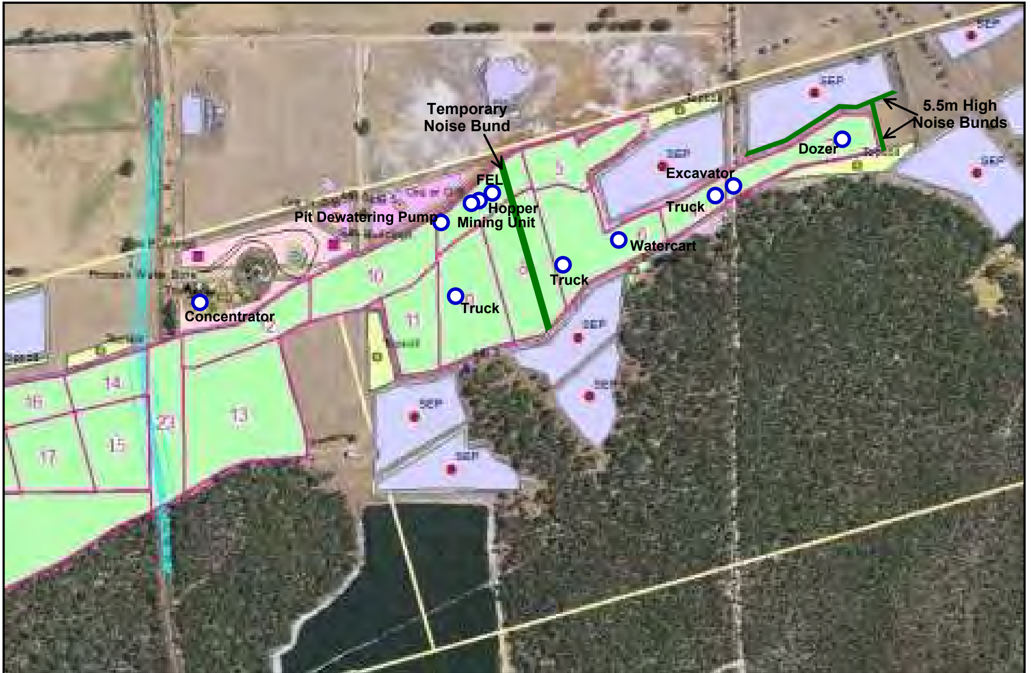
Figure 10: Assumed operating locations of the fixed plant and mobile equipment for day-time scenario 5.
