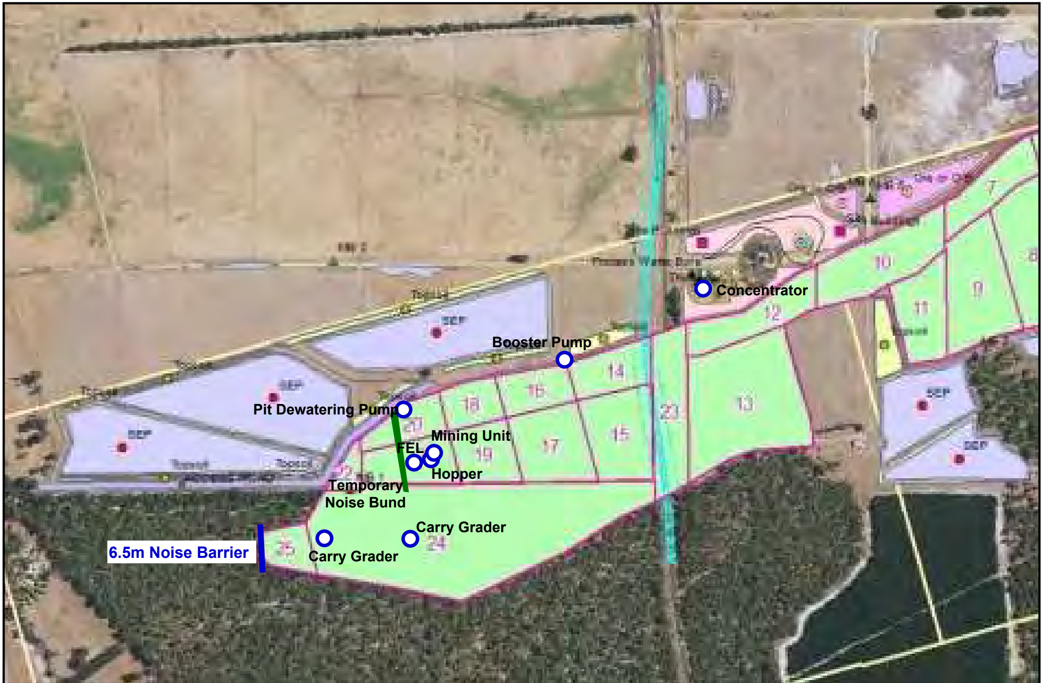
Figure 6: Assumed operating locations of the fixed plant and mobile equipment for day-time scenario 3.
