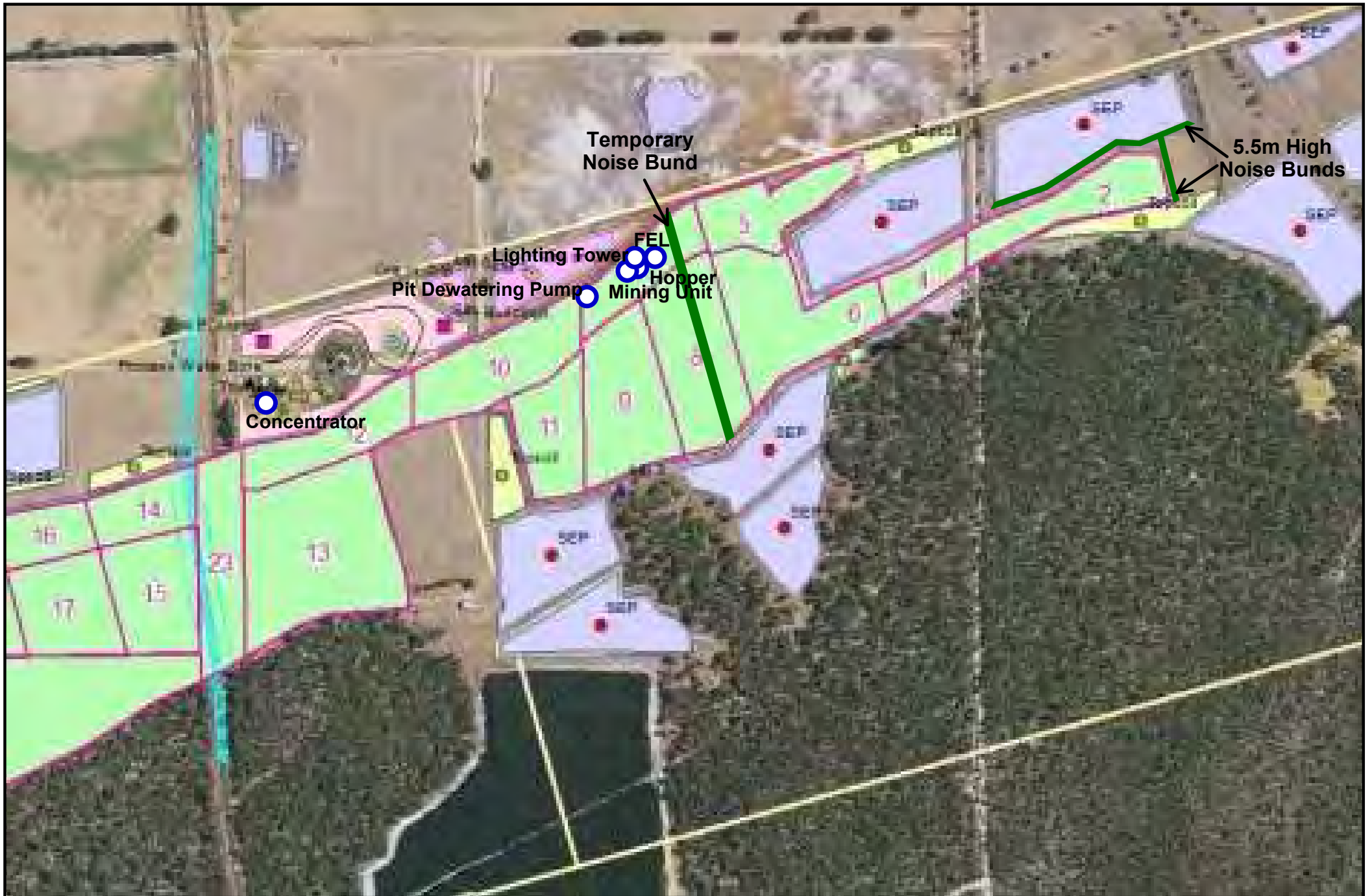
Figure 11: Assumed operating locations of the fixed plant and mobile equipment for night-time scenario 5.
