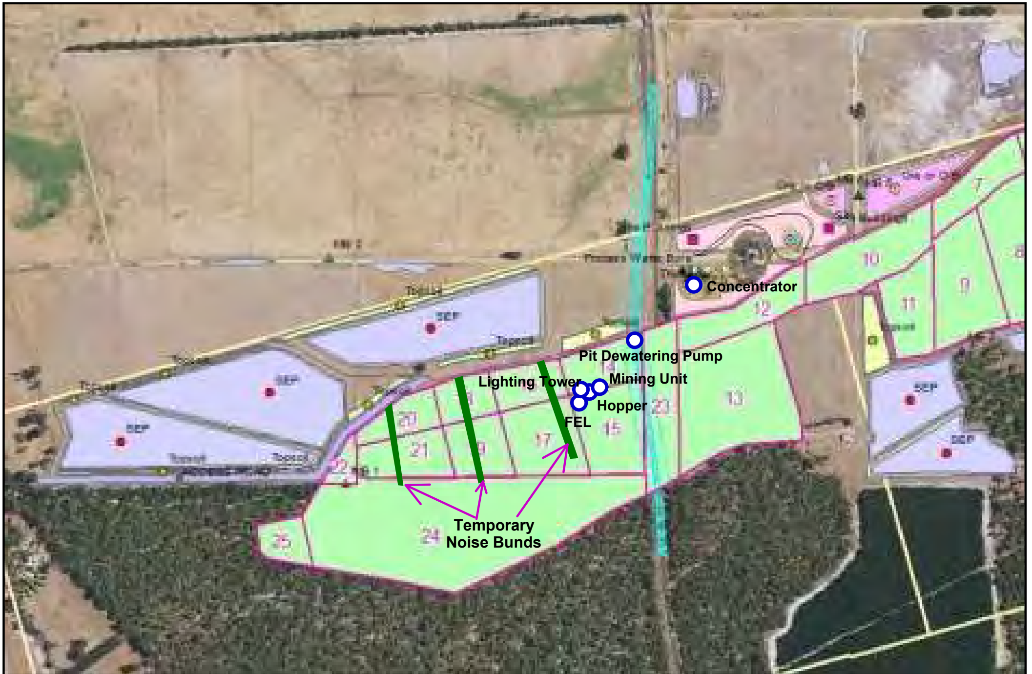
Figure 5: Assumed operating locations of the fixed plant and mobile equipment for night-time scenario 2.
