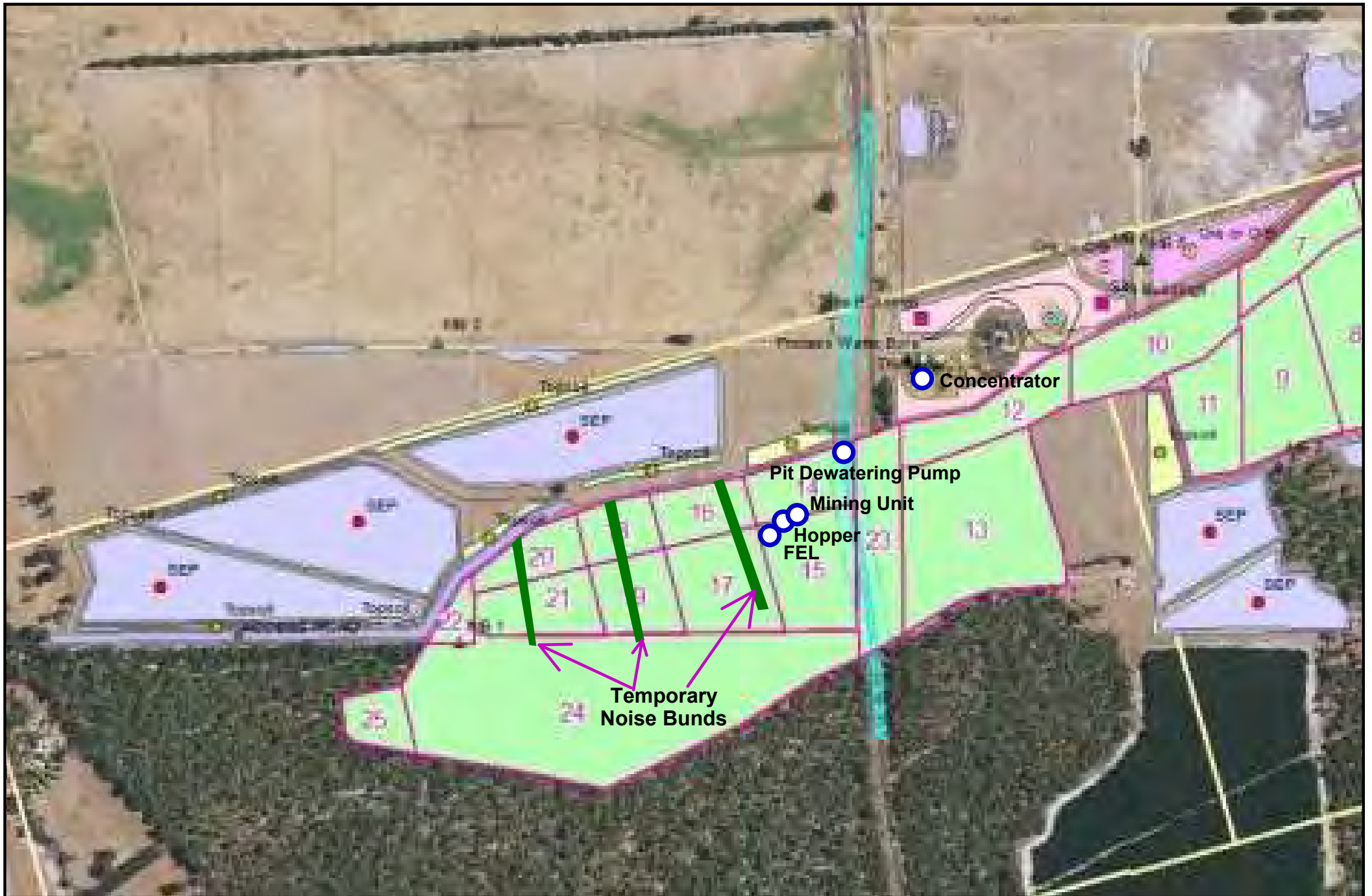
Figure 4: Assumed operating locations of the fixed plant and mobile equipment for day-time scenario 2.
