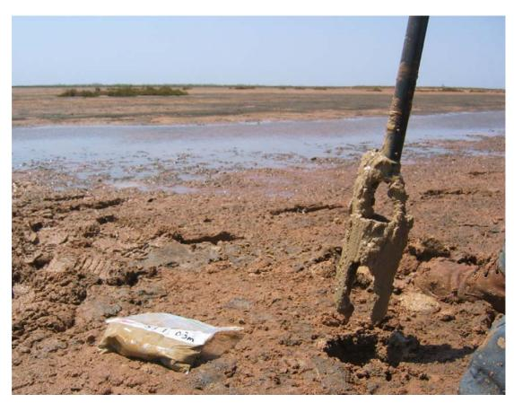
Figure 2.7 Hand augering to obtain soil samples to a depth of 2.6 m
