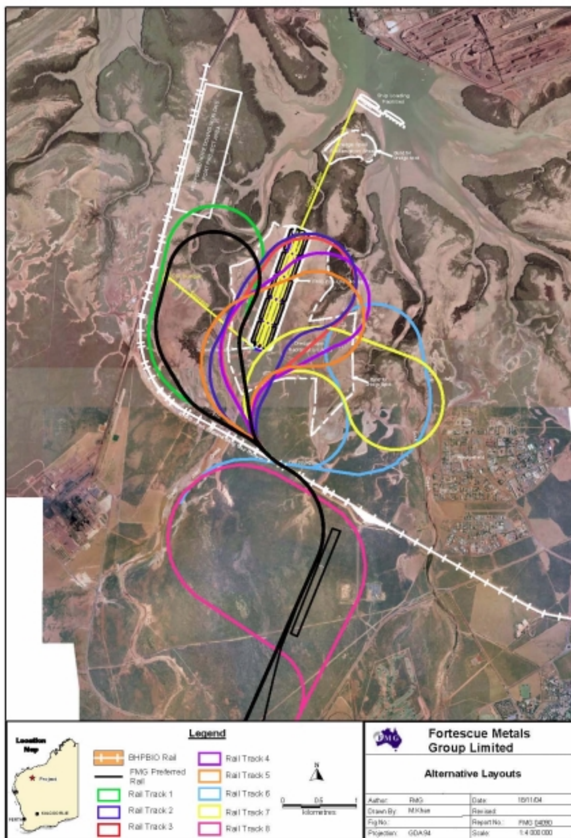
Figure 8 Possible layouts of rail loop and FMG's preferred option
