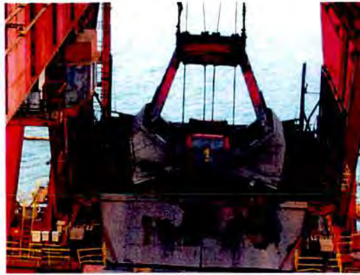
Plate 4.5 Grab Discharging Coal into Receival Hopper at Oita
