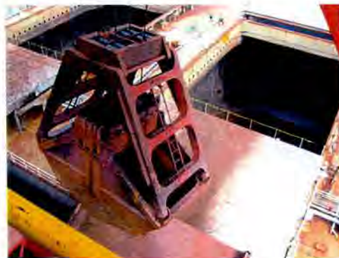
Plate 4.1 Grab Unloader at Kakogawa (the deflector plate to catch spillage is shown directly below the grab.)
