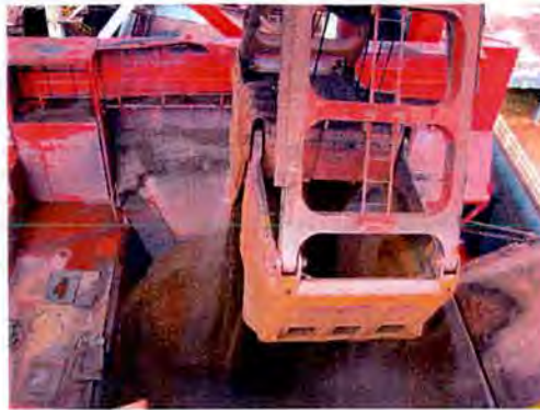
Plate 4.2 Grab Discharging Lump Ore into Receival Hopper at Kakogawa (water spray can be seen at left of grab).
