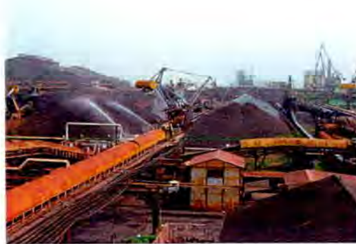
Plate 4.4 Water Sprays on Ore Stockpiles at Wakayama
