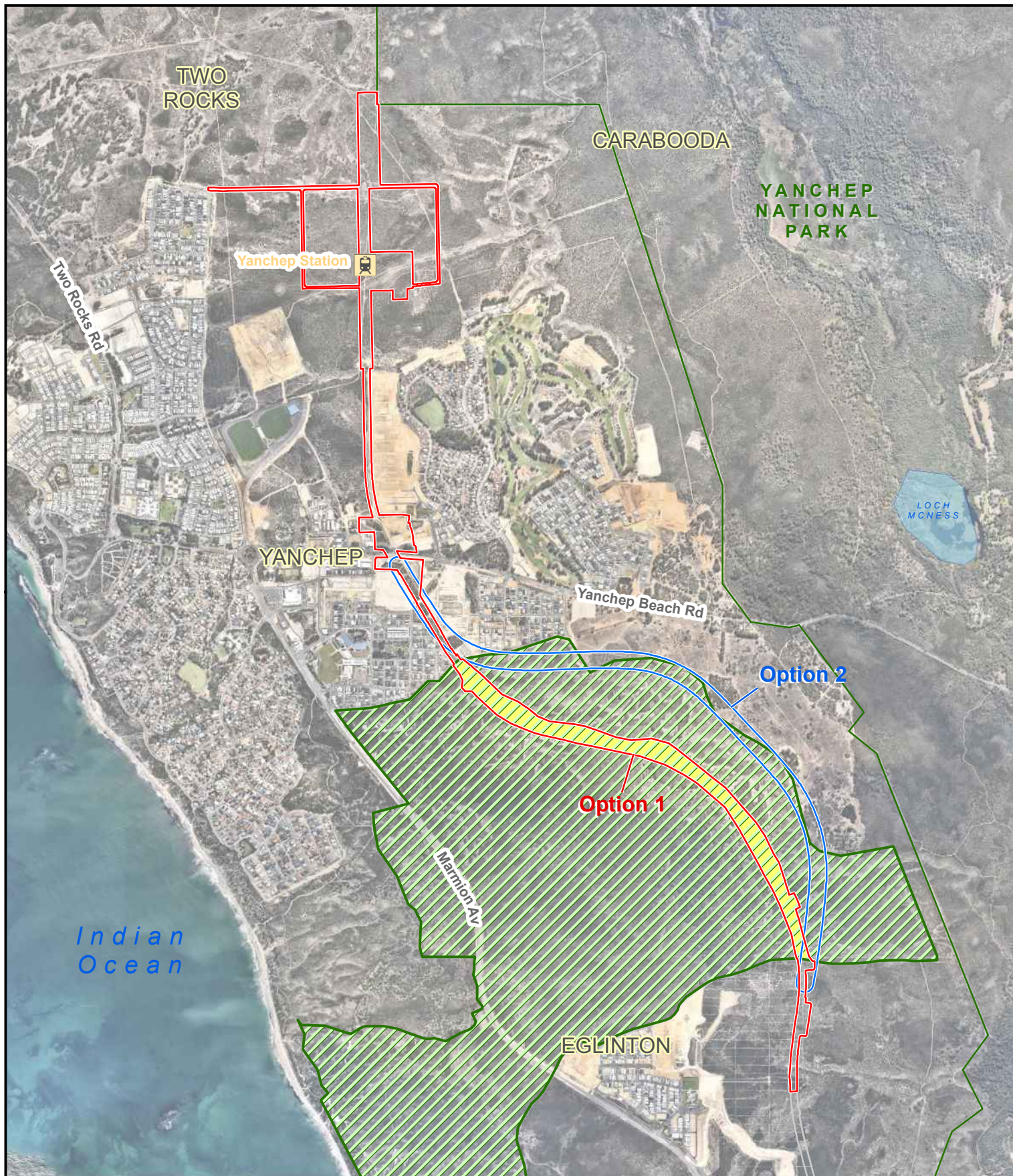
Yanchep Rail Extension (Part 2) Figure 2-1 Alternative Alignment
