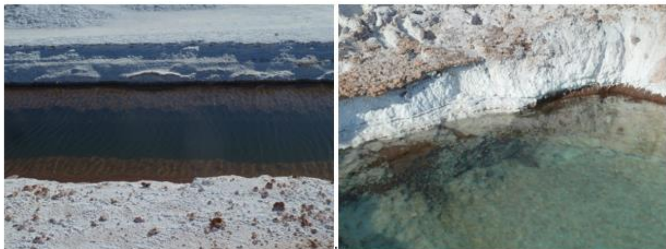
Figure 4-11: Trial brine trenches, showing low turbidity of water (Lake Disappointment, Oct 2018)
