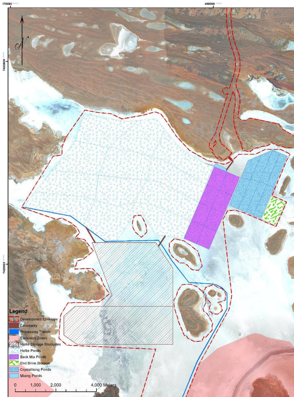
Figure 2-6: On-playa infrastructure – pond and halite stockpile detail
