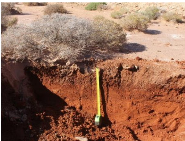
Figure 2-32: Soil profiles showing rooting depths on the playa (left) and dune soils (right)
