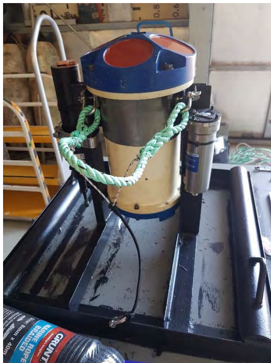
Figure 2 Loggers and ADCP setup pre-deployment for Parking (left) and Launchway (right)
