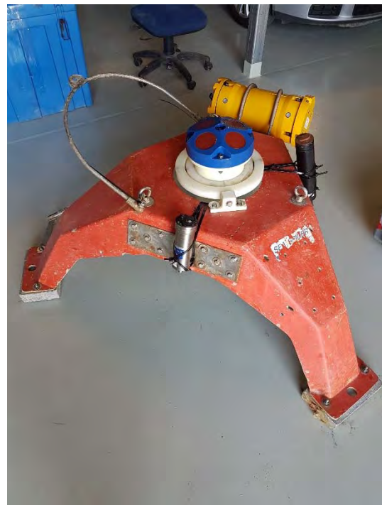
Figure 2 Loggers and ADCP setup pre-deployment for Parking (left) and Launchway (right)
