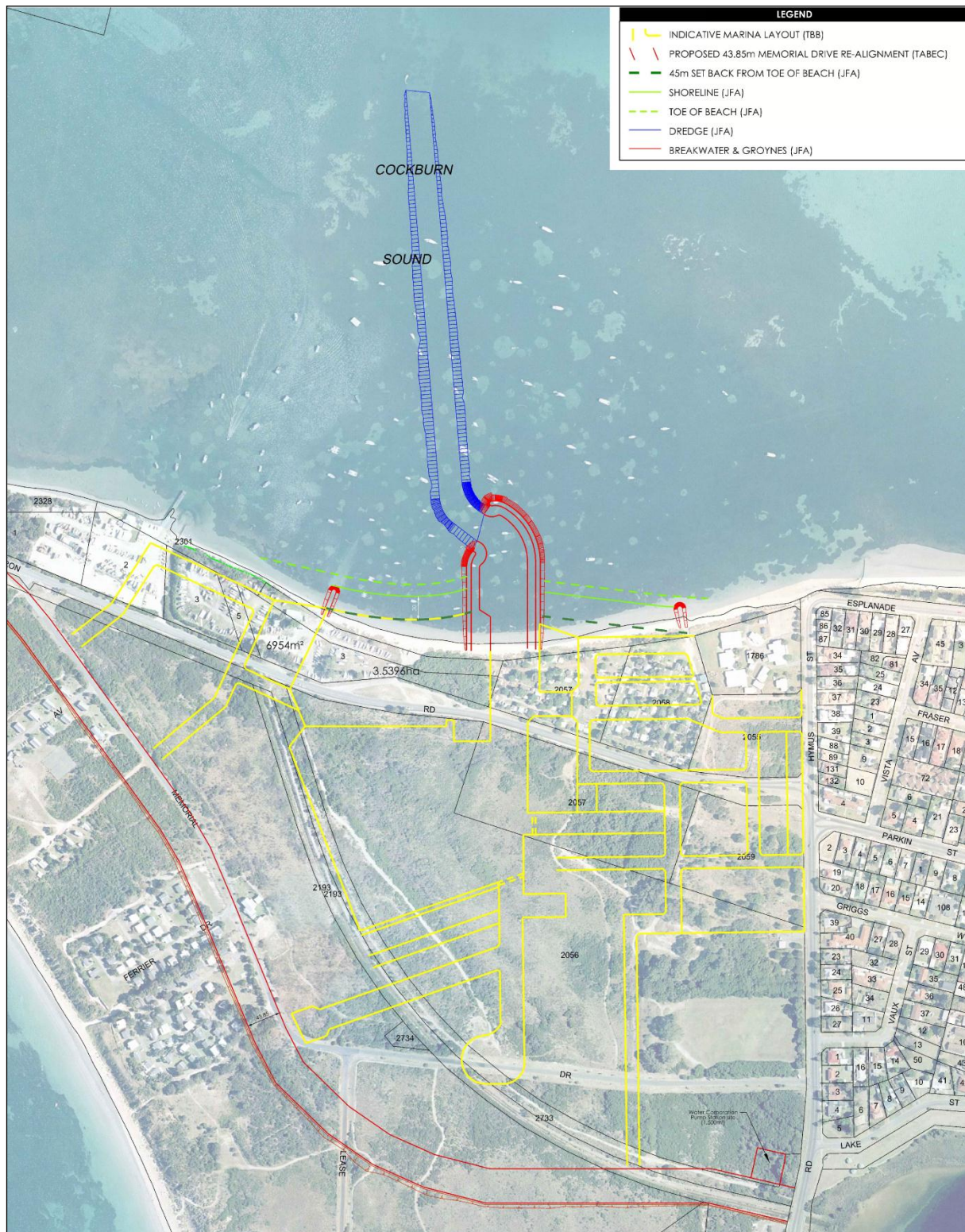
Figure 1-1 Project layout drawing showing proposed entrance channel (blue), breakwaters (red) and marina layout (yellow). Drawing provided by Cedar Woods.
