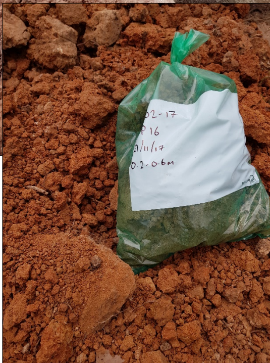
Test pit TP 16 – 2.8m termination. TOPSOIL and gravelly ALLUVIUM; red brown surficial top soil and white siltstone with some gravel.
