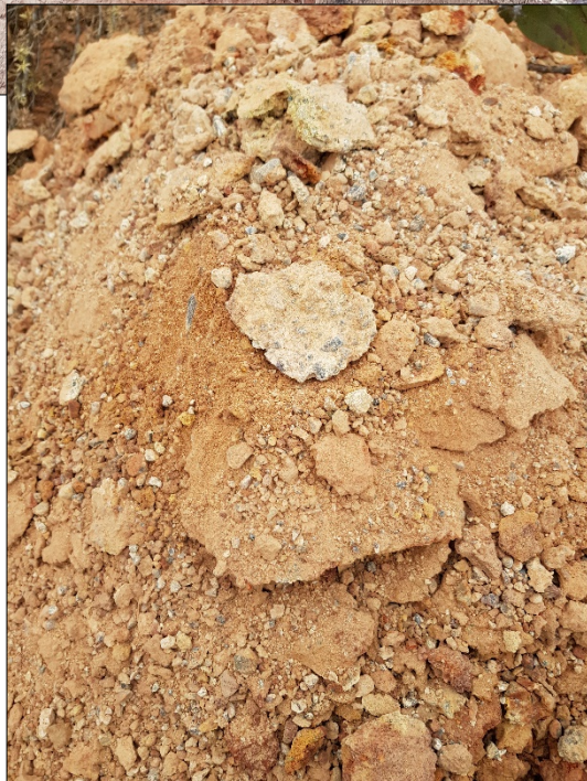
Test pit TP 20 – 1.3m refusal. TOPSOIL into lateritic ALLUVIUM, gravelly and conglomeritic.
