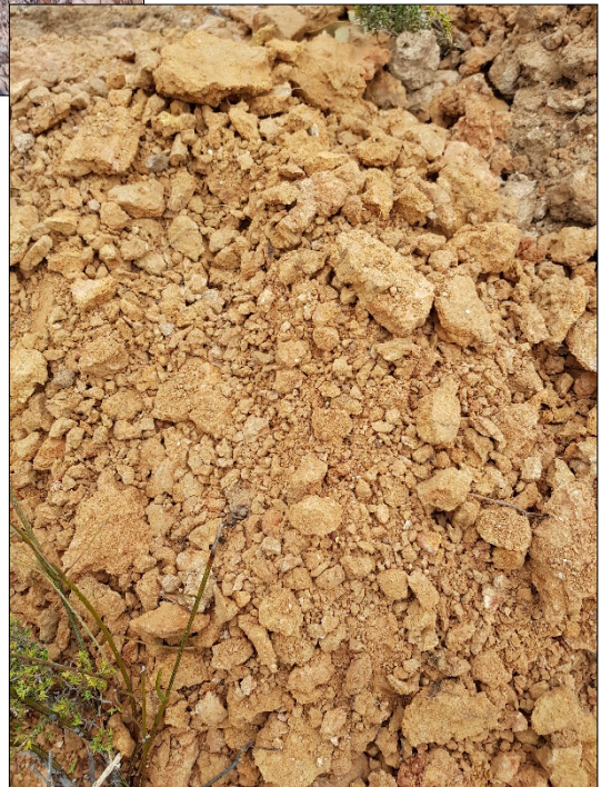
Test pit TP 20 – 1.3m refusal. TOPSOIL into lateritic ALLUVIUM, gravelly and conglomeritic.
