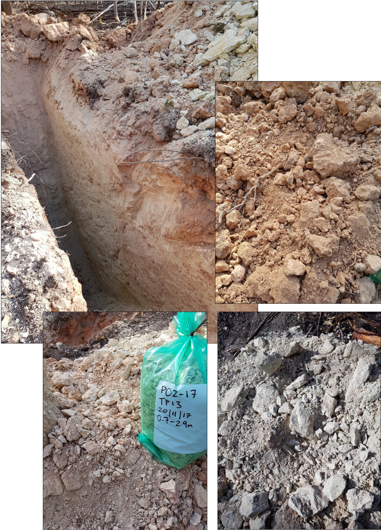
Test pit TP 13 – 2.9m terminated, 3 soil horizons. TOPSOIL and ALLUVIUM; brown grey surficial top soil and white siltstone with some red mottling.
