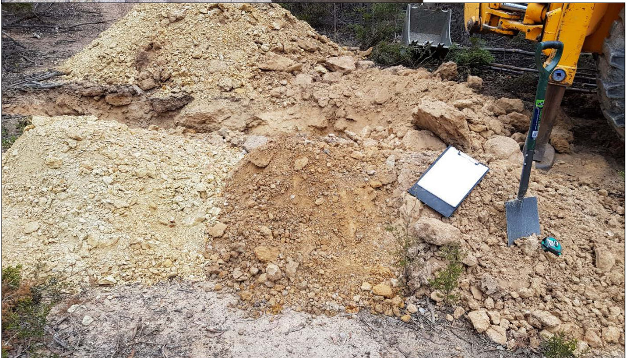
Test pit TP 17 – 2.7m termination. TOPSOIL (right) grading into ALLUVIUM, white siltstone (left).
