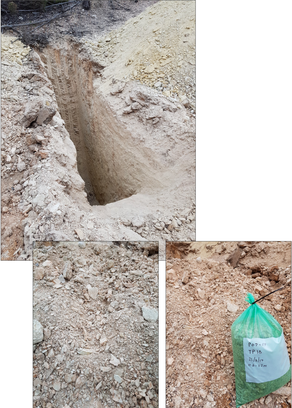
Test pit TP 18 – 2.7m termination. TOPSOIL (right) grading into ALLUVIUM, white siltstone (left).
