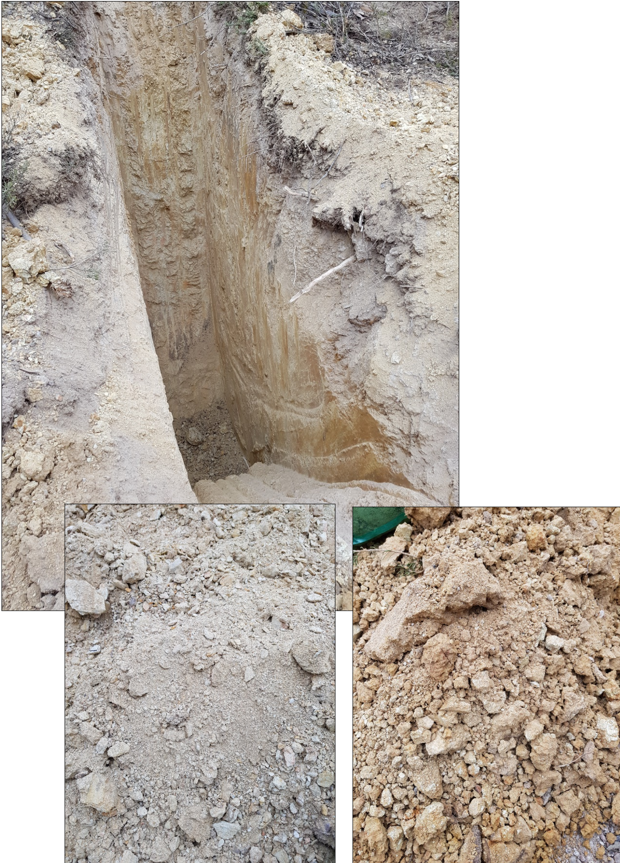
Test pit TP 19 – 2.8m termination. TOPSOIL grading into ALLUVIUM, white siltstone.
