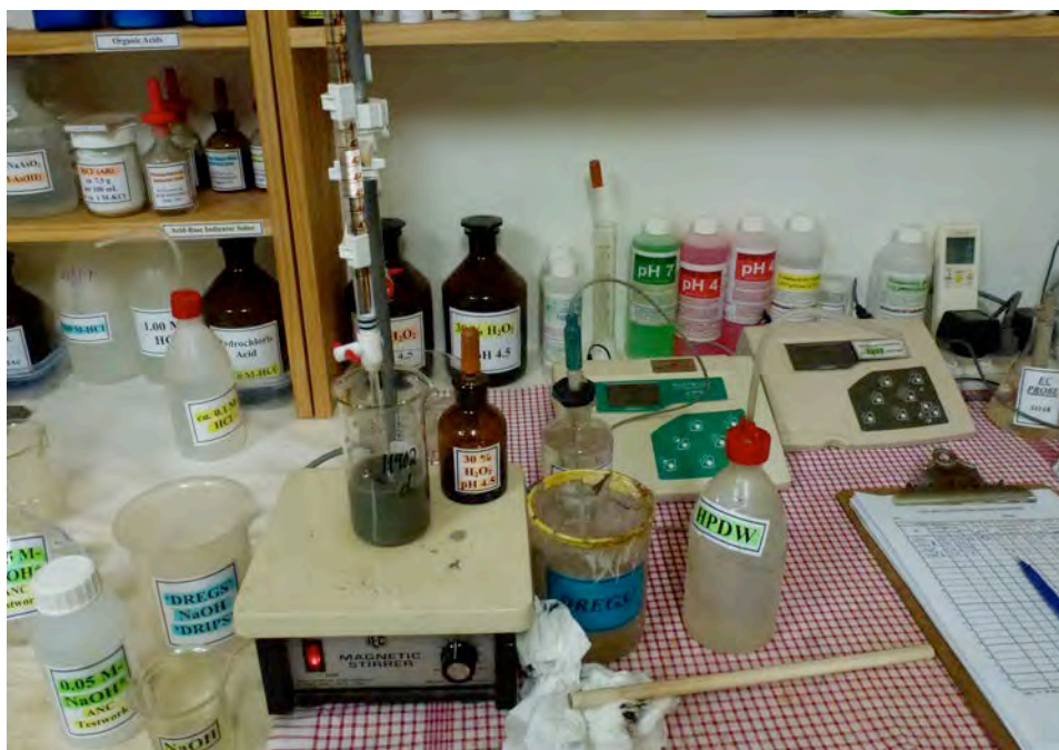
PLATE 2: Acid-Neutralisation-Capacity (ANC) testing.
