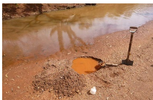
Plate 1. Collection of the hyporheic sample from WARUS5, using the Karaman-Chappuis method. Photo by WRM ©
