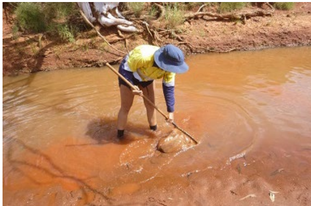
Plate 2. Sampling for macroinvertebrates using a 250 \mu\text{m} mesh FBA d-frame dip net. Photo by WRM ©.
