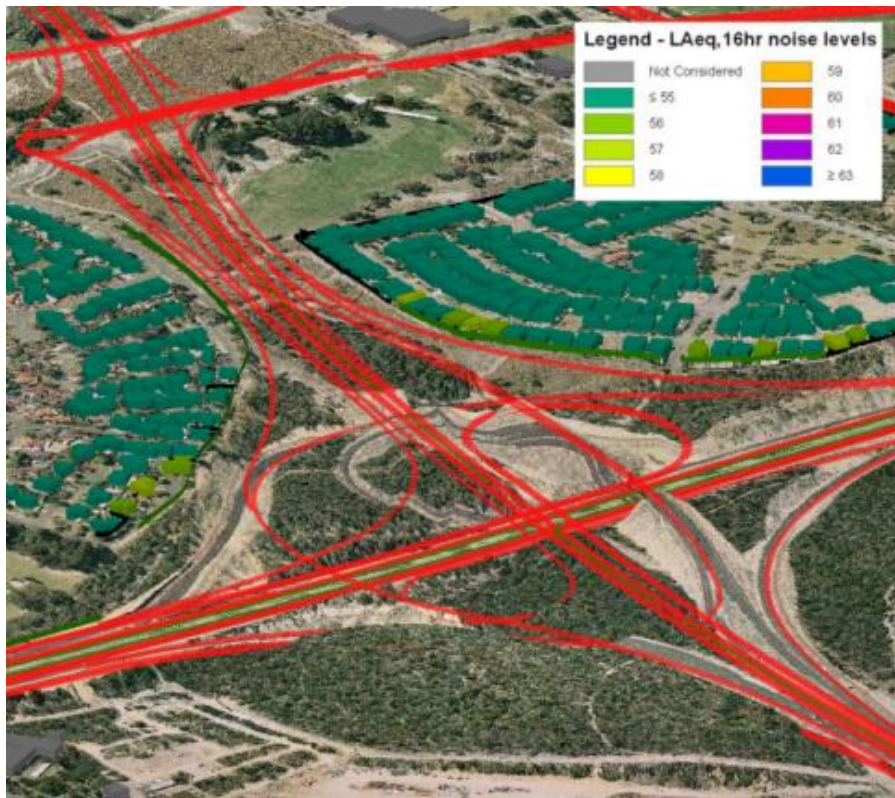
Figure 31 Proposed barrier layout – Kwinana Fwy interchange (north-easterly view)
