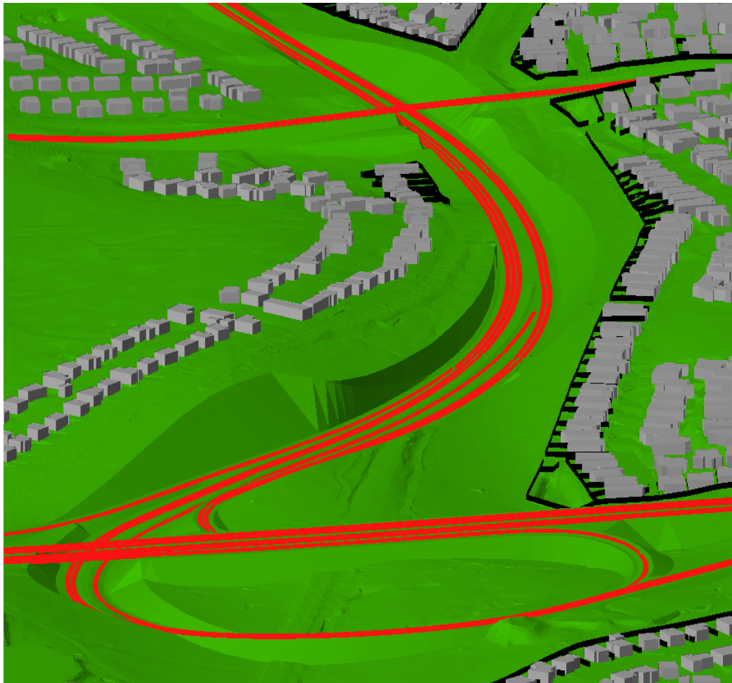
Figure 9 Proposed vertical road alignment – Stock Rd Interchange to Sudlow / Coolbellup Overpass (easterly view)
