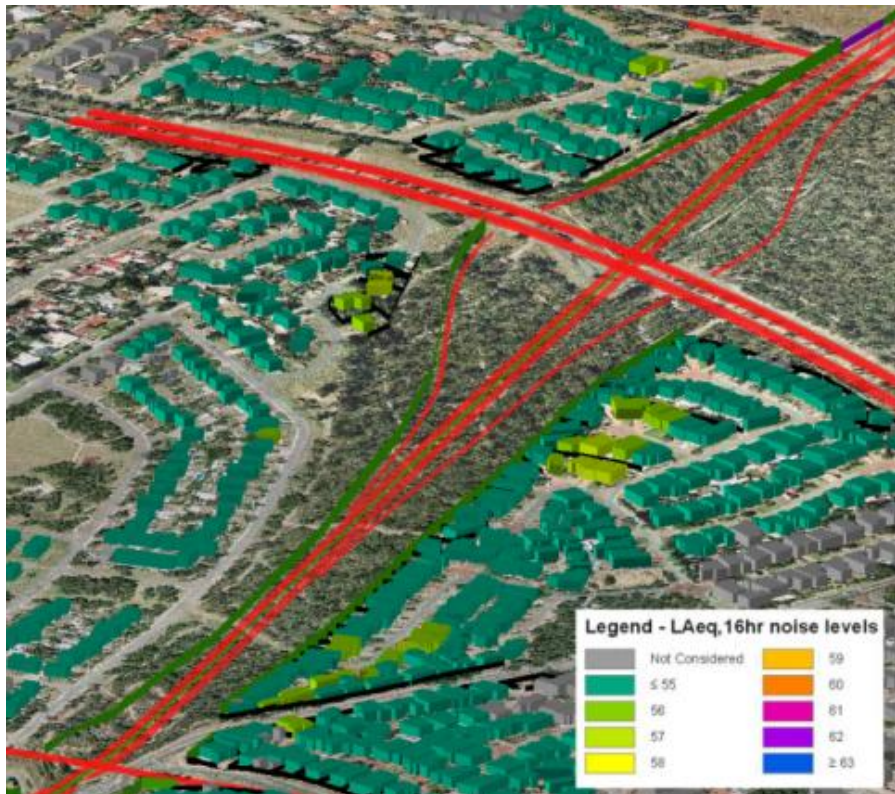
Figure 29 Proposed barrier layout – Sudlow / Coolbellup overpass to Progress Drive
