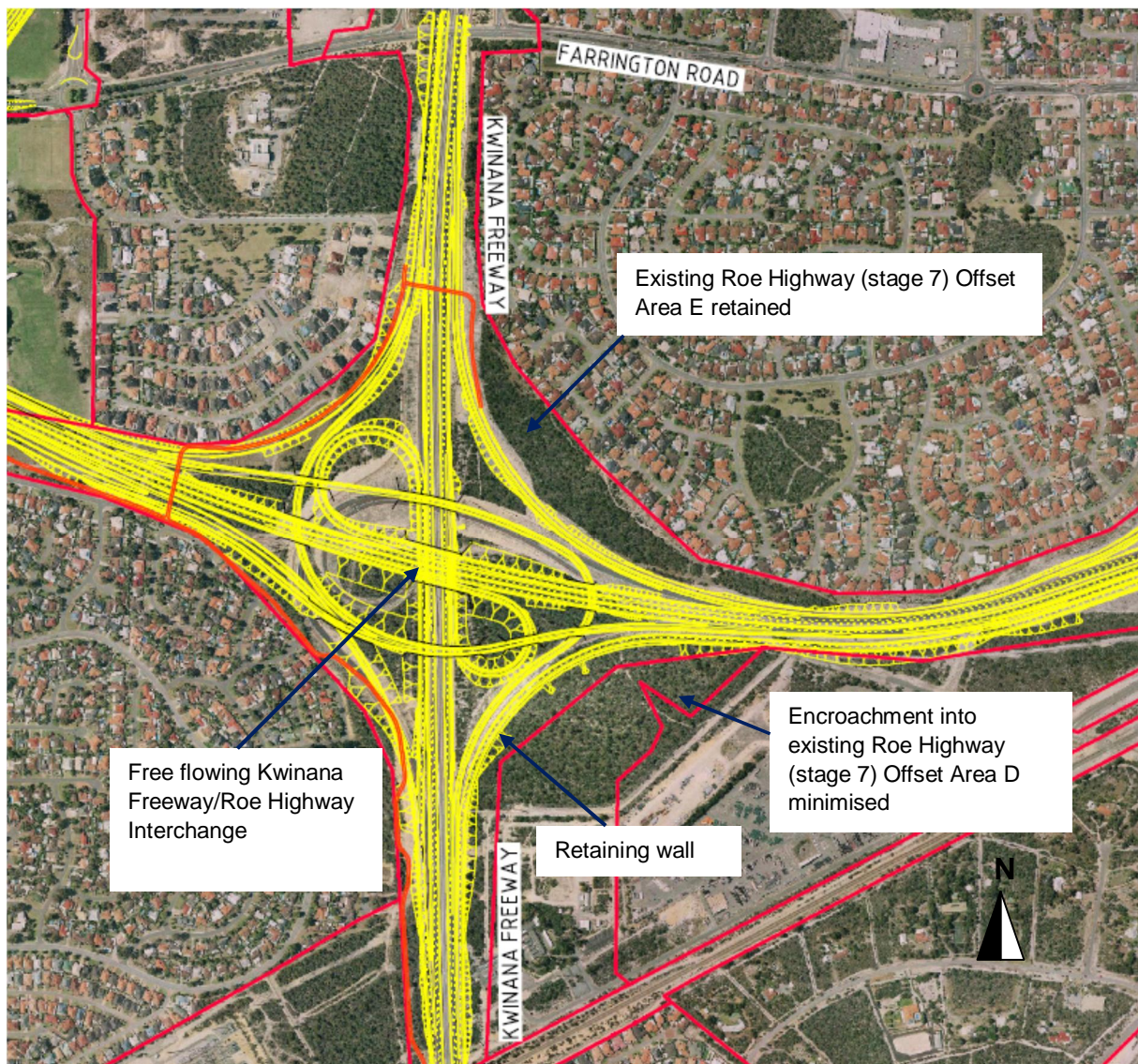
Figure 5: Roe Highway Extension Preferred Option, Free Flowing Kwinana Freeway/Roe Highway Interchange
