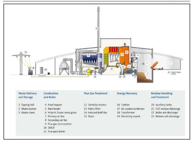
Figure 3 Generic schematic of Waste to Energy plant recently completed by HZI
