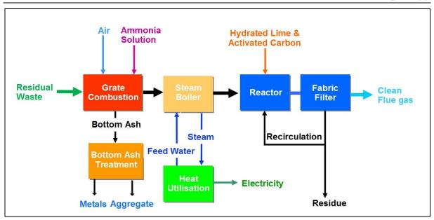
Figure 4 Bloc Flow Diagram of grate-combustion, steam boiler and flue gas cleaning system
