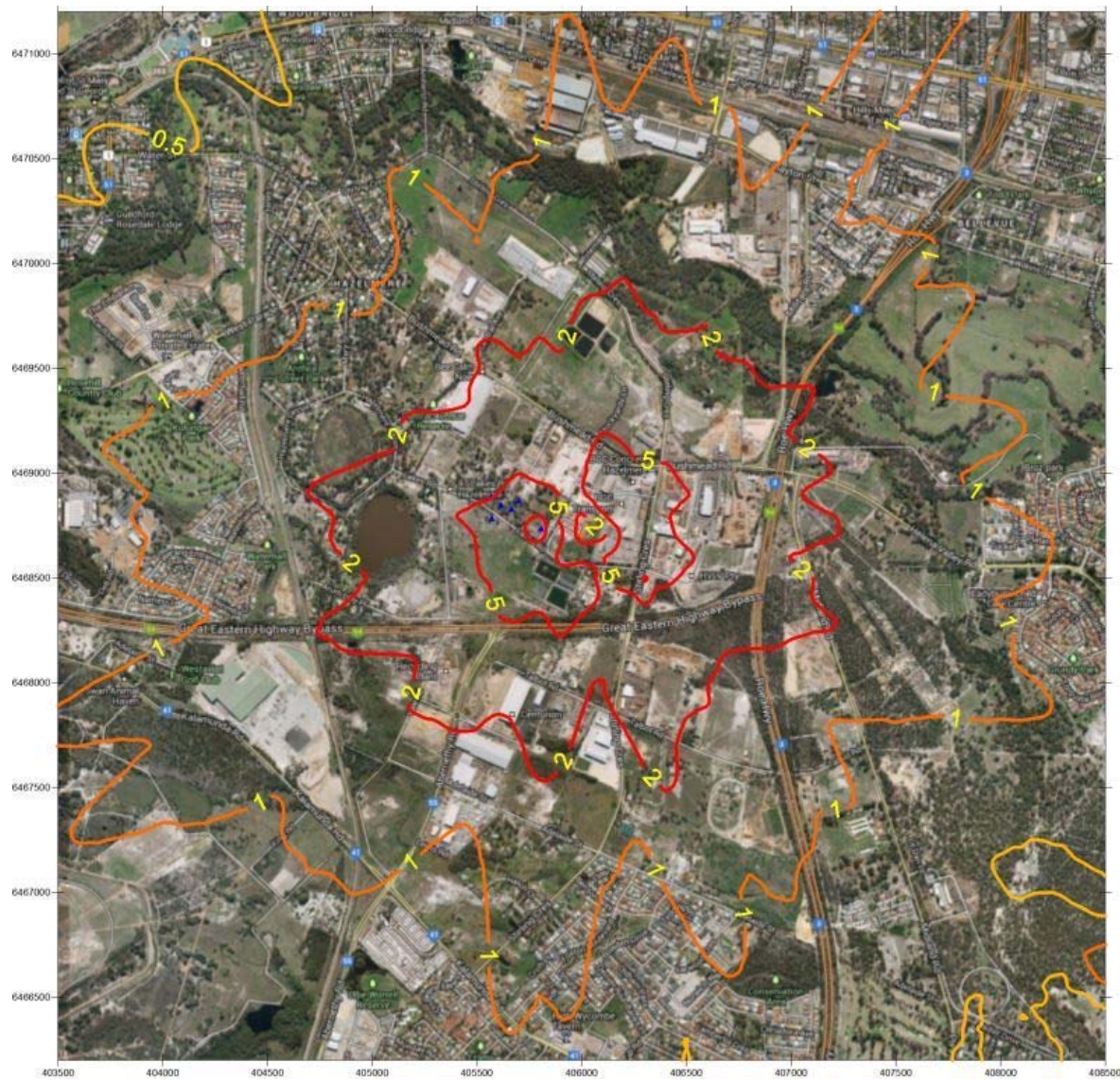
Figure 179: Bypass Operations - GLC Cu (ng/m³) Maximum 8-Hourly
