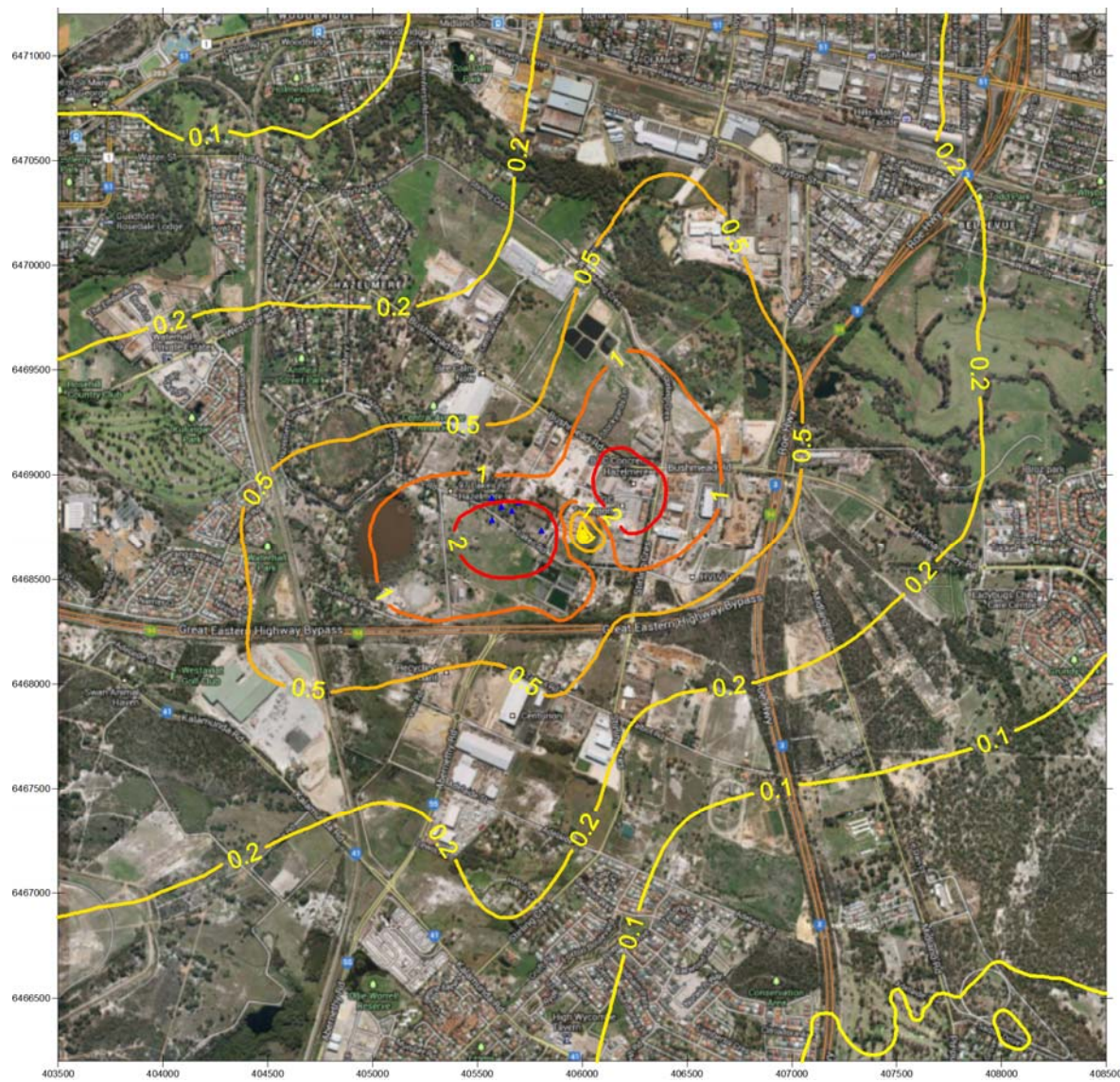
Figure 198: Bypass Operations - GLC Mn ( \text{fg}/\text{m}^3 ) Maximum Hourly
