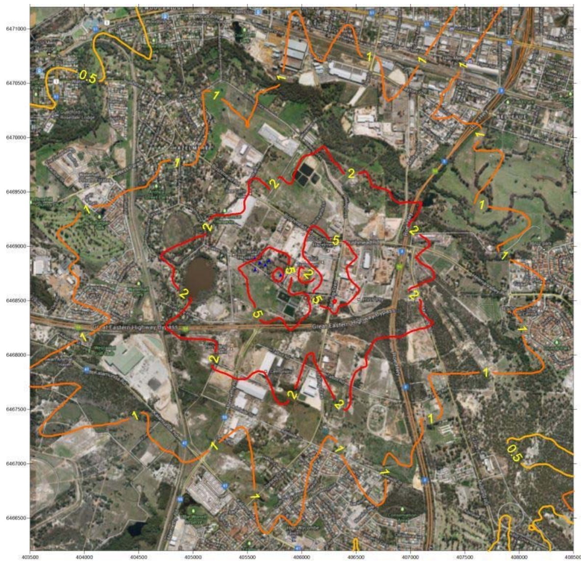
Figure 199: Bypass Operations - GLC Mn ( \text{fg}/\text{m}^3 ) Maximum 8-Hourly
