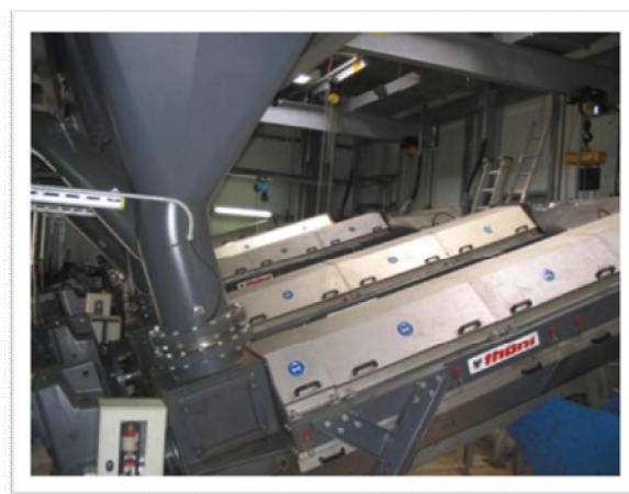
Figure 8 Screw Press for Dewatering Digestate
