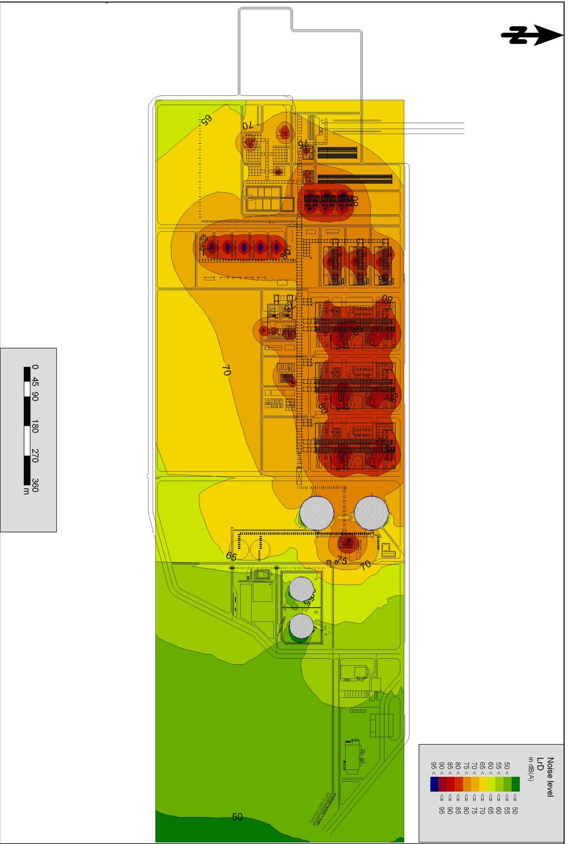
**Figure 11.1: Noise Contours within the Gas Treatment Plant and at Plant Boundary**
