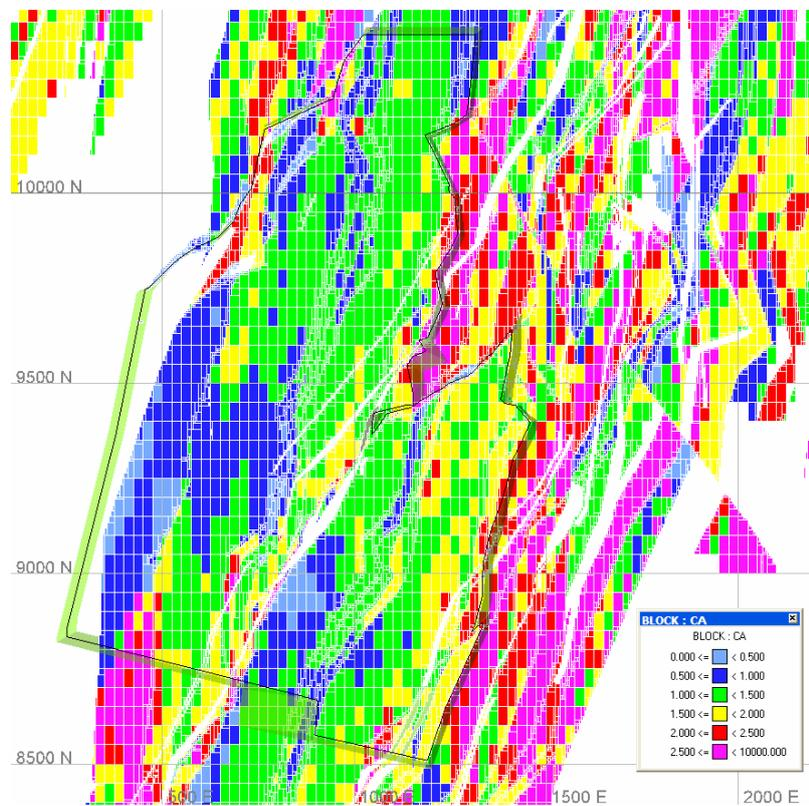
Figure 22: CaO (wt%) Distribution for SIP Pit Shell at -50 m RL
