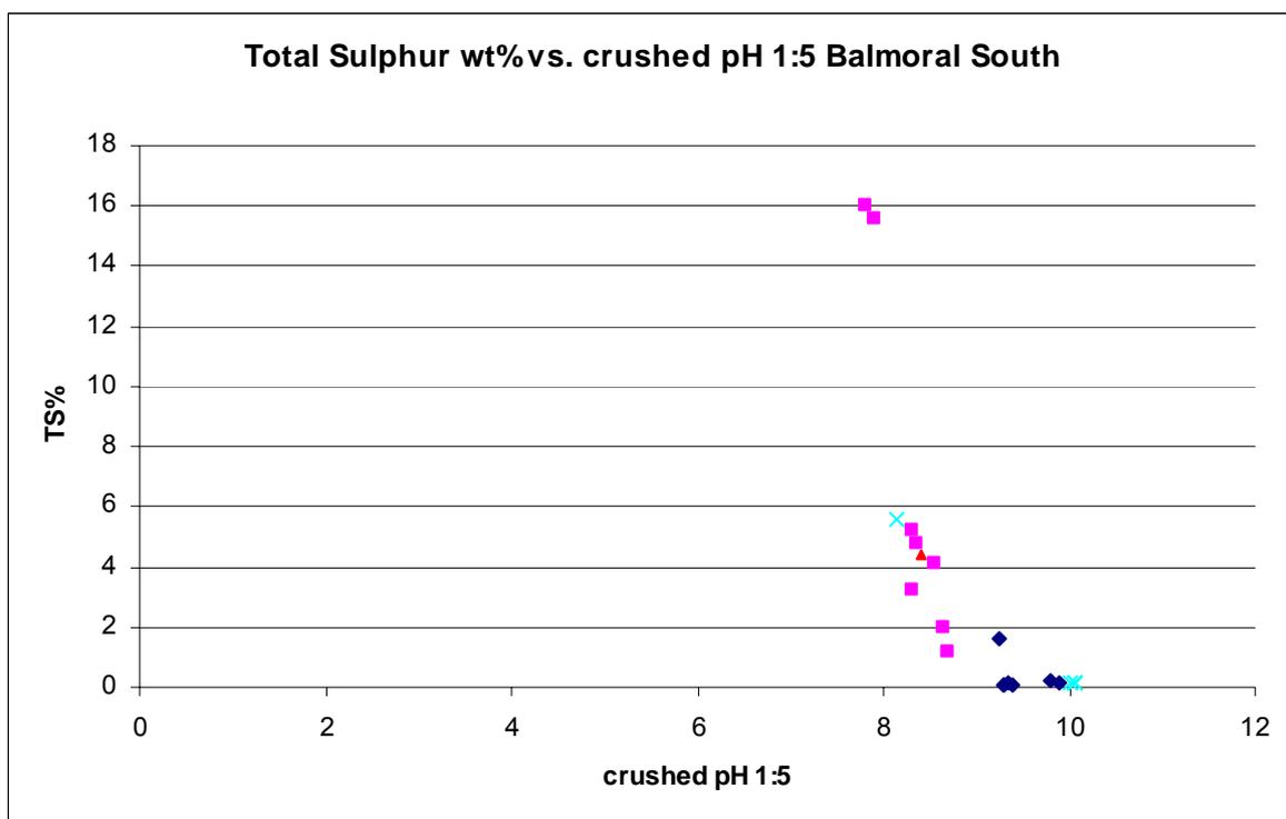
Figure 4: Total Sulphur wt % vs. Crushed pH<sub>1:5</sub>
