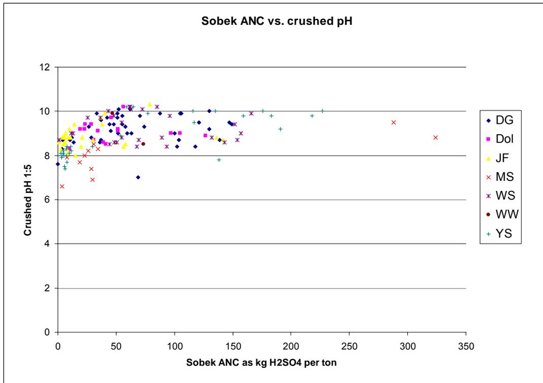
Figure 3: Sobek ANC vs. Crushed pH<sub>1:5</sub>
