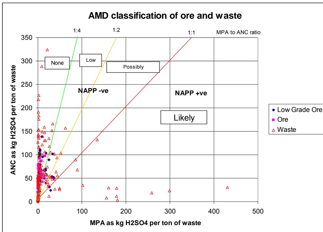
Figure 9: ABA Classification of Samples Using Davies Tube Recovery Test to Define Economic Classification of the SIP Samples According to Price 1997.
