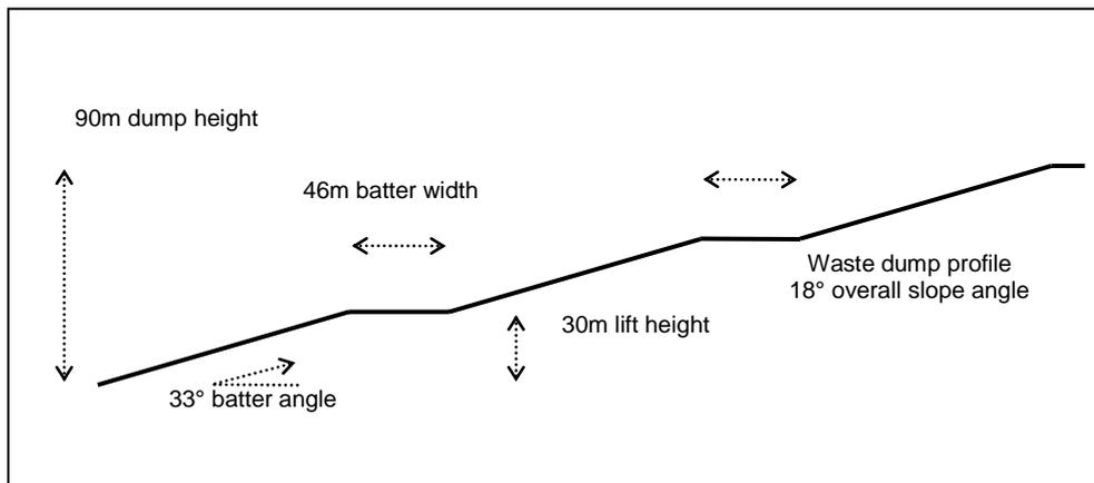
**Figure Error! No text of specified style in document.-1: Waste Disposal Facility Design Profile**
