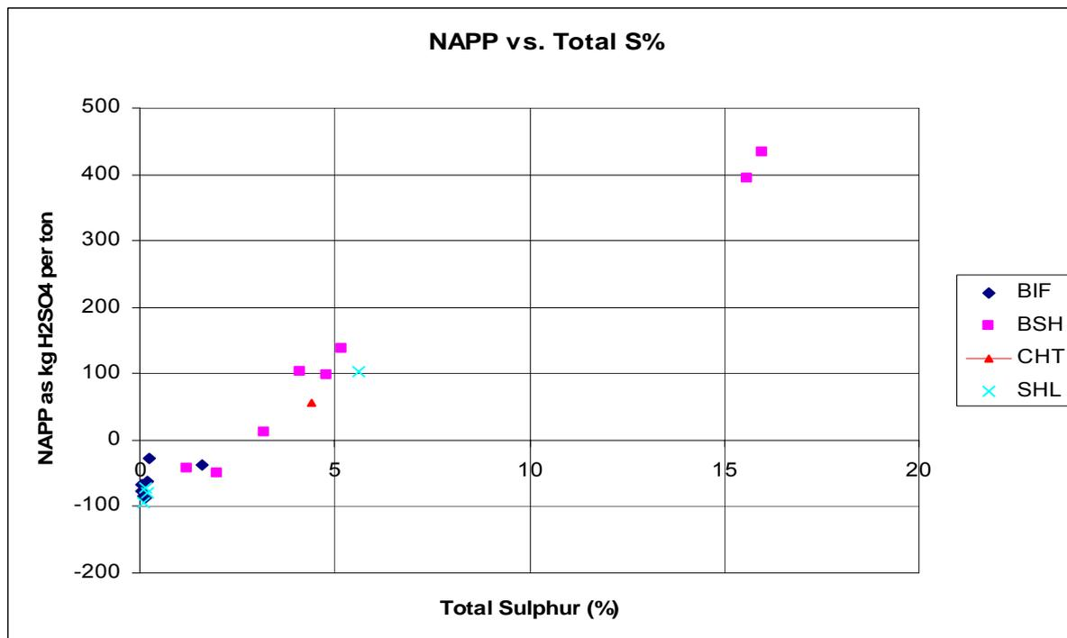
Figure 12: NAPP vs Total Sulphur for Balmoral South
