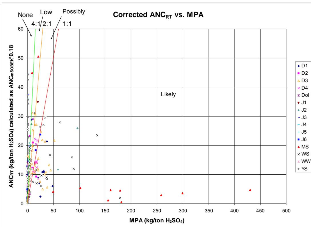
Figure 18: Calculated  $ANC_{RT}$  plotted against MPA according to Price (1997)
