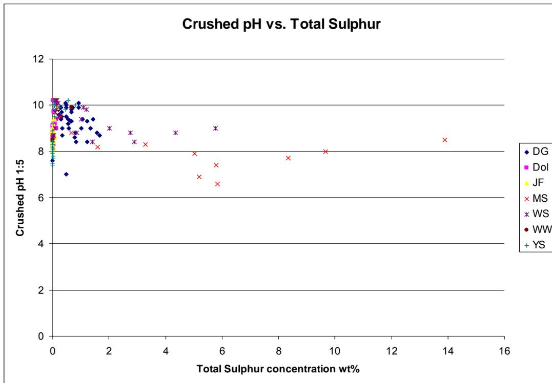
Figure 2: Total Sulphur wt% vs. Crushed pH<sub>1:5</sub>
