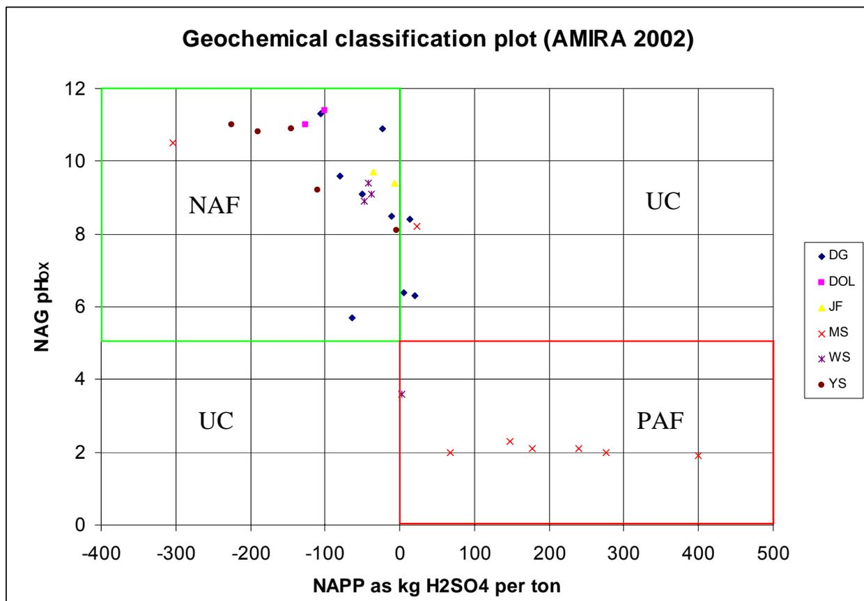
Figure 13: NAG vs. NAPP Plot for Selected SIP Samples
