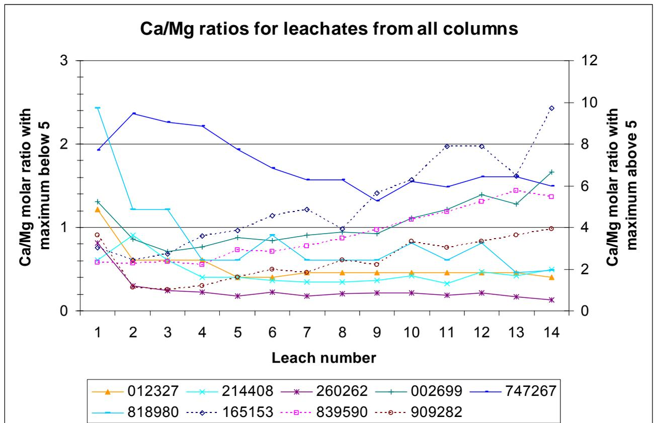
Figure 19: Ca/Mg Molar Ratios for Kinetic Leach Columns Over the Test Period, with Trends Exceeding 3 Plotted with Open Symbols and Dotted Lines on the Secondary Y Axis
