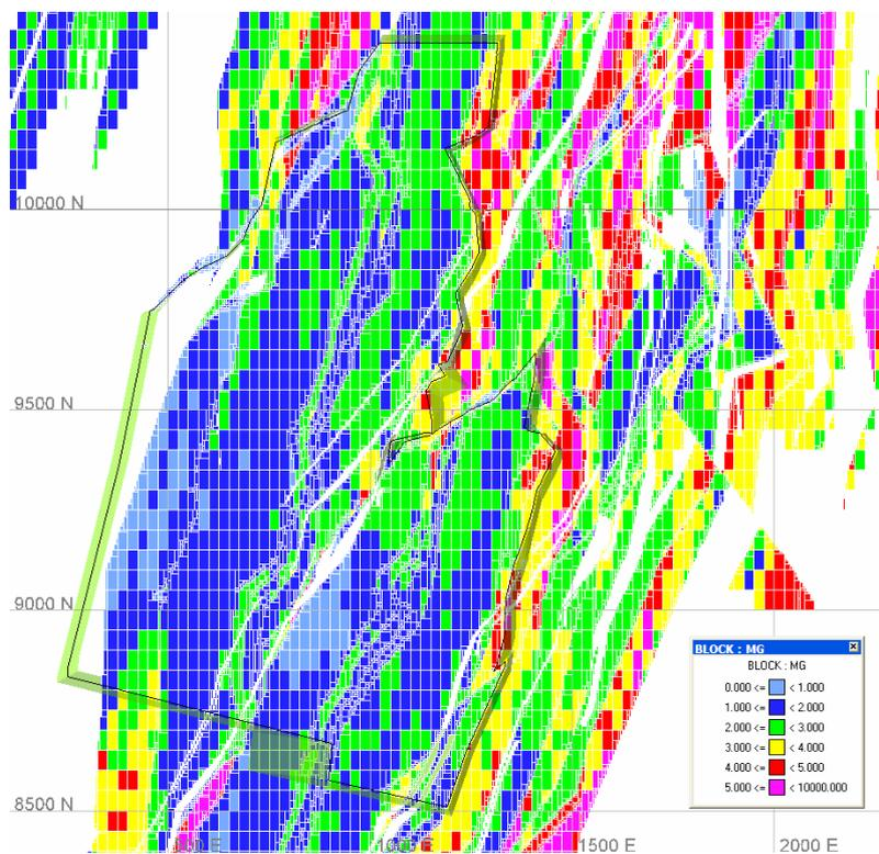
Figure 24: MgO (wt%) Distribution for SIP Pit Shell 23 at -150 m RL
