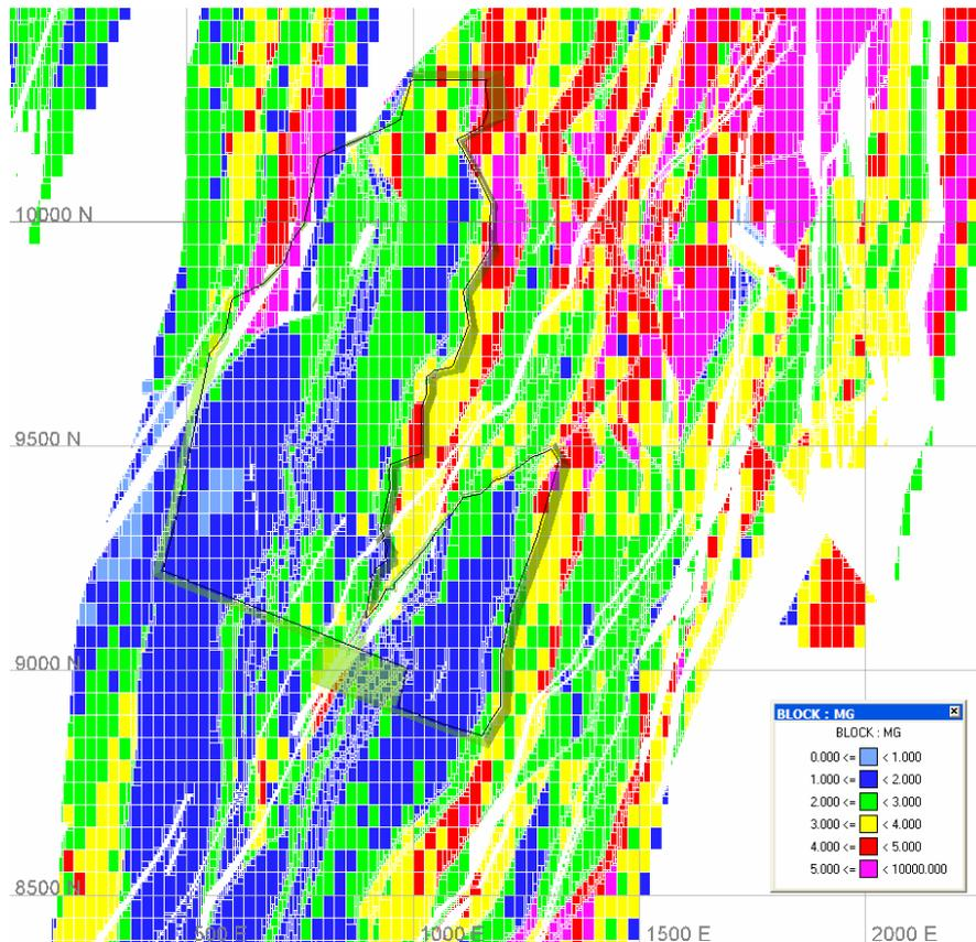
Figure 25: MgO (wt%) Distribution for SIP Pit Shell 23 at -150 m RL
