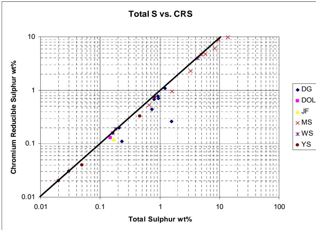
Figure 15: CRS wt% vs. TS wt%
