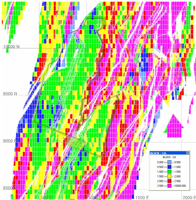
Figure 23: CaO (wt%) Distribution for SIP Pit Shell 23 at -150 m RL
