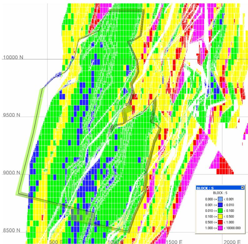
Figure 20: Sulphur Distribution (wt%) for SIP Pit Shell at -50 m RL
