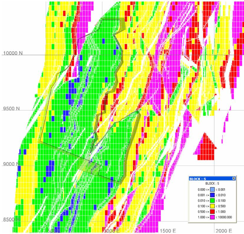
Figure 21: Sulphur Distribution (wt%) for SIP Pit Shell 23 at -150 m RL
