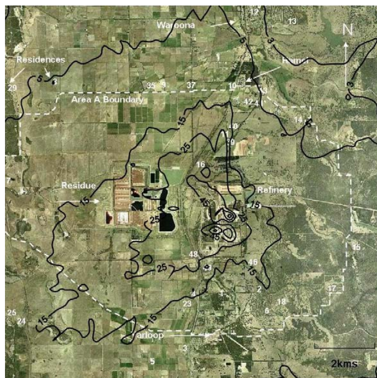
Figure 21: Peak (99.9th percentile) 3-minute odour concentrations for the existing refinery. Contours in odour units/m 3 .
