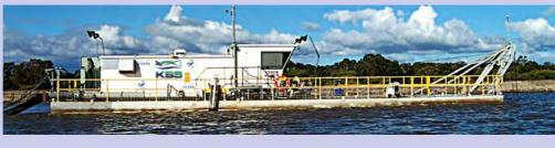
The dredge operates using a hydraulically driven cutter head to disturb the material which in turn is then sucked up by a pump which is situated on board.
