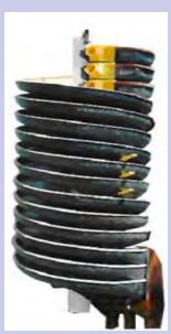
Spirals are used at Kemerton to remove heavy minerals such as Iron, Ilmenite Zircon etc from our silica sand product.
