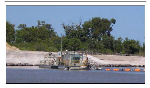
Plate 3. Final dredging to 7–10 m of quartzite ore.
