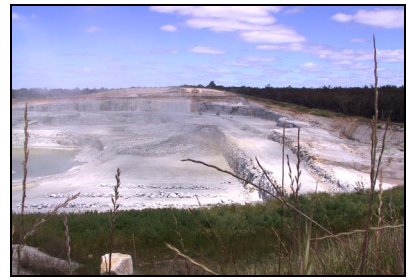
Plate 8 After the blast conducted on 8 October 2002. All rock landed within the pit as the blast was designed to force the material inwards towards the pit.
