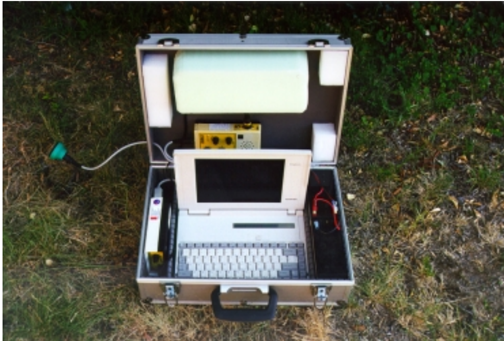
Plate 1. The ultrasonic bat detector units used to record bat activity.
