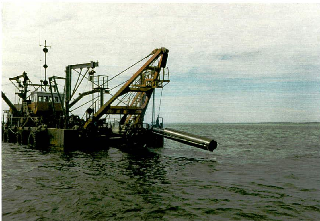
Plate 1: The water jet suction dredge 'Success'.
