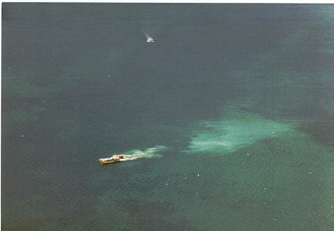
Plate 2: Dredge in operation. Downstream turbidity is intermittent and limited in area.
