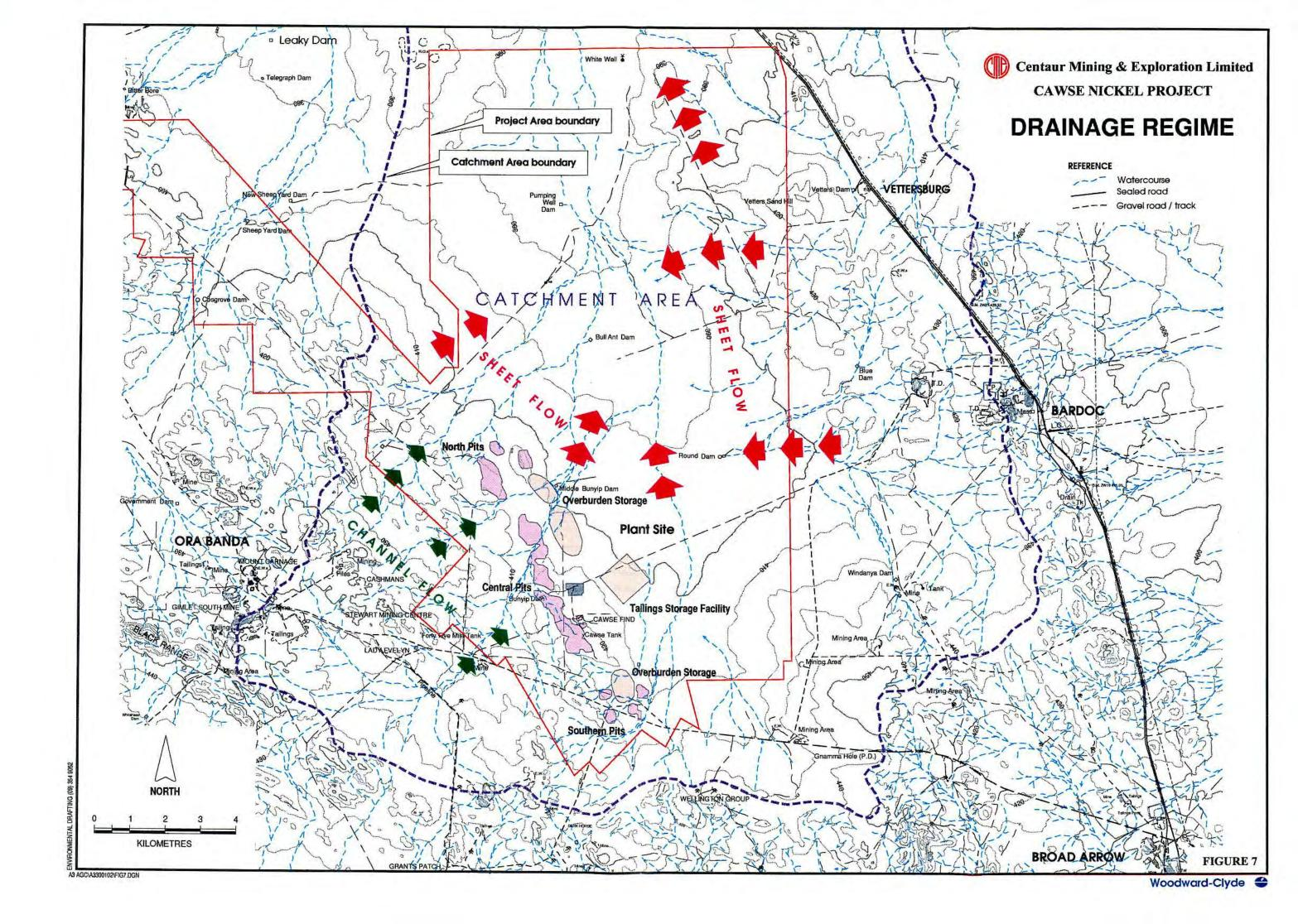
Most of the Project area including the mine, processing plant and tailings storage facility is located at higher points in the landscape where natural drainage lines are well defined.
