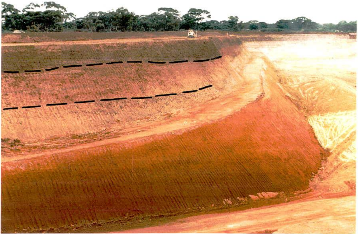
Stratification in the open pit at Kanowna Belle results from a deep soil profile (3 m) overlying a transitional zone (centre) and weathering zone at base.
