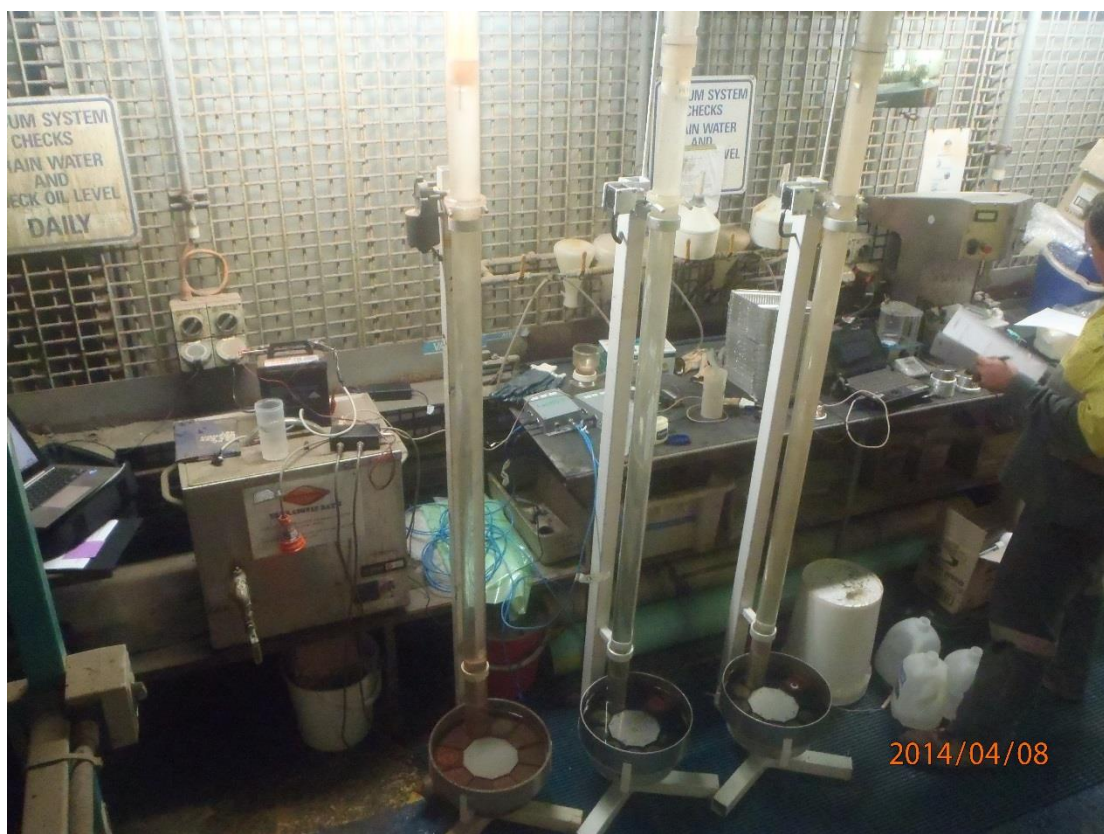
Figure 9: Landloch's automated settling columns deployed on site in support of field based rainfall simulation.
