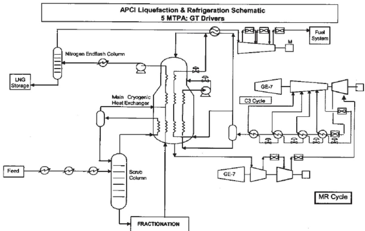
Pre-cooling duty and cooling of mixed refrigerant is provided by the propane circuit which consists of a 4 stage, single casing compressor and 10 propane kettles operating at 2 to 17.6 barg and down to -36 °C. The propane refrigerant compressor flowrate is 2.1 million kg/hr of propane. Major equipment in the propane circuit includes the propane condenser (aircooler, 173 MW, 15.5 m x 203 m long) and LLP Propane suction drum (7.4 m ID x 9.8 m T/T).
