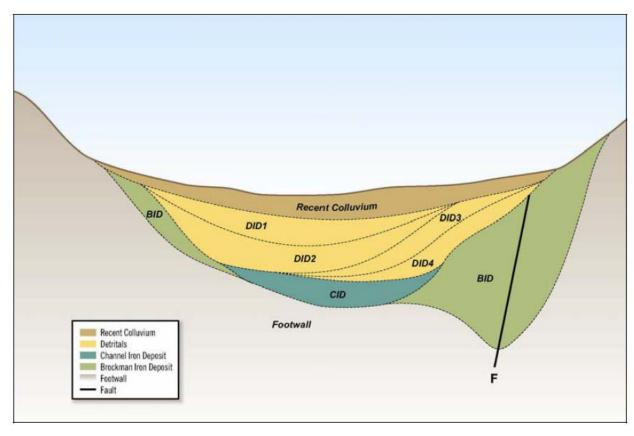
Figure 2: Schematic Cross-Section of Pilbara Style CID Mineralisation (Worley Parsons, 2012)
