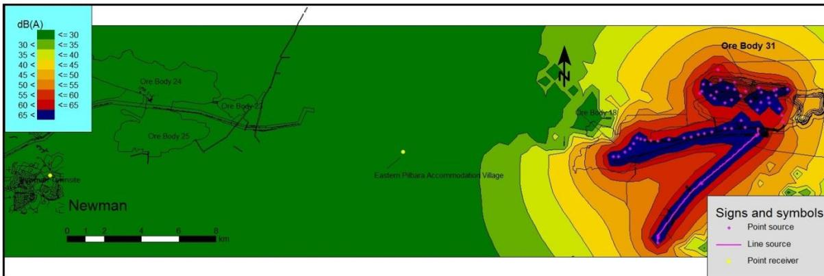
*Figure 4-1 Scenario 5 – Noise Model Overview - Noise Contour Map*
