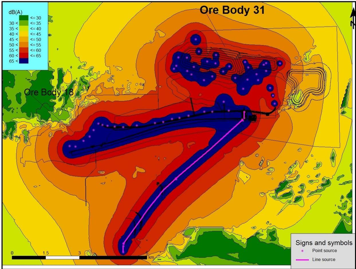
Figure 4-2 Scenario 5 – Noise Contour Map of Plant
