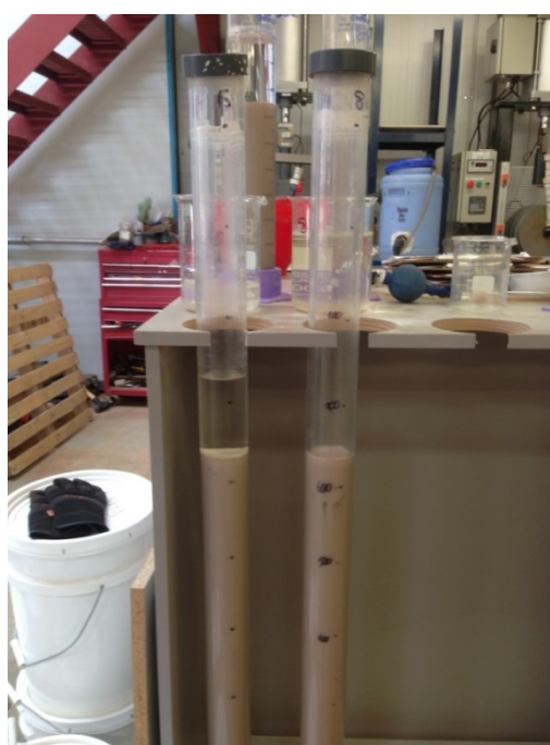
Figure 7: FHG tailings undrained and top drained tests (left); bottom drained and top/bottom drained tests (right).
