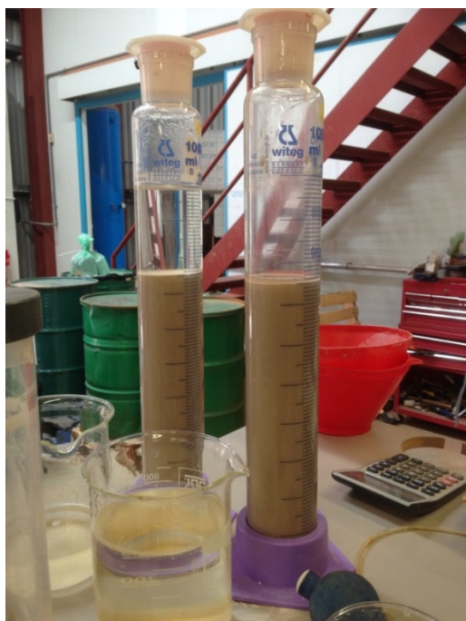
Figure 7: FHG tailings undrained and top drained tests (left); bottom drained and top/bottom drained tests (right).
