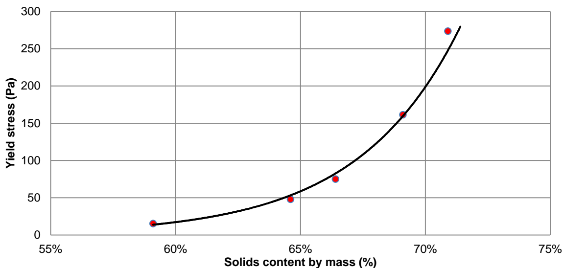
Figure 17: Yield stress against percentage of solids
